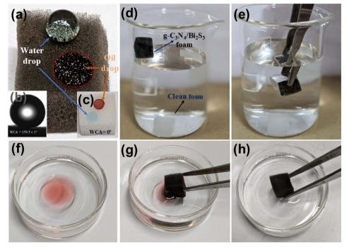
Fig. 6 (a) The water and oil droplets on the  $g-C_3N_4/Bi_2S_3$  foam surface. Inset (b): WCA of  $g-C_3N_4/Bi_2S_3$  foam; inset (c): water and oil droplets on a pure melamine foam. (d and e) photographs of the  $g-C_3N_4/Bi_2S_3$  foam and a pure melamine foam immersed in water. (f–h) Present sequential photographs demonstrating the oil removal process from water using the  $g-C_3N_4/Bi_2S_3$  foam.
