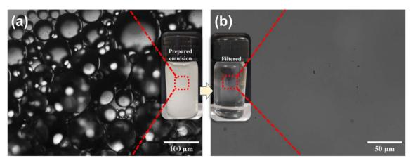
Fig. 10 Photograph of the prepared oil-in-water emulsion (a) before and (b) after separation.
