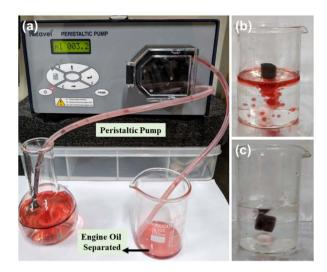
Fig. 9 The separation of oil from water using the g-C<sub>3</sub>N<sub>4</sub>/Bi<sub>2</sub>S<sub>3</sub> foam by: (a) continuous separation facilitated by a peristaltic pump, and (b and c) continuous stirring of oil in water.
