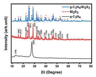
Fig. 2 XRD patterns of synthesized  $g-C_3N_4$ ,  $Bi_2S_3$ , and  $g-C_3N_4/Bi_2S_3$  nanocomposite.
