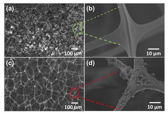
Fig. 3 FESEM images of (a and b) pure melamine foam and (c and d)  $g-C_3N_4/Bi_2S_3$  coated melamine foam at different magnifications.
