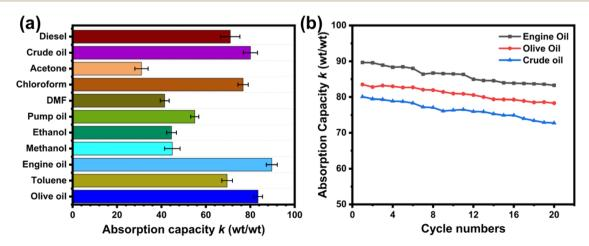
Fig. 8 (a) The absorption capacity of g-C<sub>3</sub>N<sub>4</sub>/Bi<sub>2</sub>S<sub>3</sub> foam with different organic solvents and oils. (b) Recyclability of g-C<sub>3</sub>N<sub>4</sub>/Bi<sub>2</sub>S<sub>3</sub> foam absorption using manual squeezing for oil recovery.
