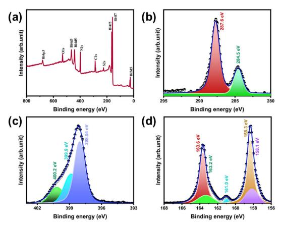
Fig. 4 XPS (a) survey scan of  $g-C_3N_4/Bi_2S_3$  foam. (b)–(d) Narrow scan XPS of  $g-C_3N_4/Bi_2S_3$  foam: (b) C 1s and (c) N 1s and (d) Bi 4f.
