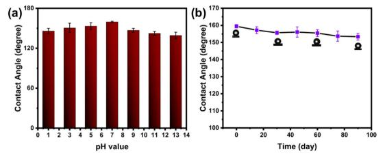
Fig. 7 (a) Stability test of the  $g-C_3N_4/Bi_2S_3$  foam after 24 h in the solutions with different pH values. (b) Variation in the WCA of  $g-C_3N_4/Bi_2S_3$  foam with exposure to air over a period of 0 to 90 days.
