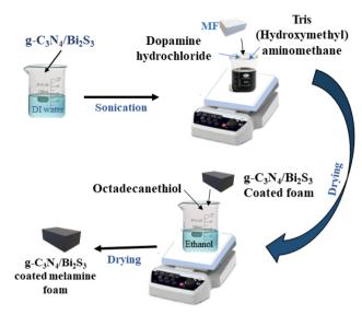
Fig. 1 Schematic diagram for the preparation of g- $C_3N_4/Bi_2S_3$  coated melamine foam.
