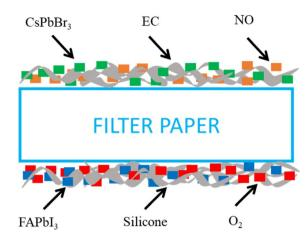
Fig. 2 Schematic structure device sensing of the  $NO-O_2$  dual gas sensor.
