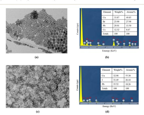
Fig. 1 (a) TEM images and (b) EDS spectra of CsPbBr<sub>3</sub> perovskite QDs, (c) TEM images and (d) EDS analysis result for FAPbl<sub>3</sub> perovskite QDs.
