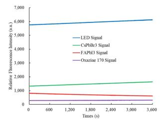
Fig. 9 Photostability of the optical dual sensor.
