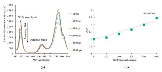
Fig. 5 (a) Response of optical dual sensor at different NO concentrations and (b) Stern-Volmer plot.
