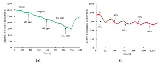
Fig. 8 Dynamic response of optical dual sensor for (a) NO and (b) O<sub>2</sub> sensor.
