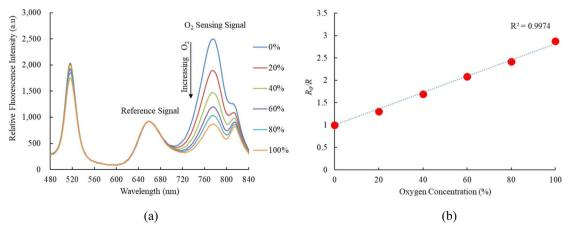
Fig. 6 (a) Response of optical dual sensor at different O<sub>2</sub> concentrations and (b) Stern-Volmer plot.
