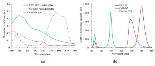
Fig. 4 (a) Absorption and (b) emission spectrum of FAPbl<sub>3</sub>, CsPbBr<sub>3</sub> QDs, and oxazine 170.
