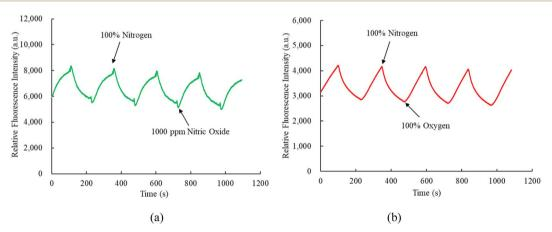
Fig. 7 Response and recovery time of the optical dual sensor for (a) NO and (b) O<sub>2</sub> sensor.
