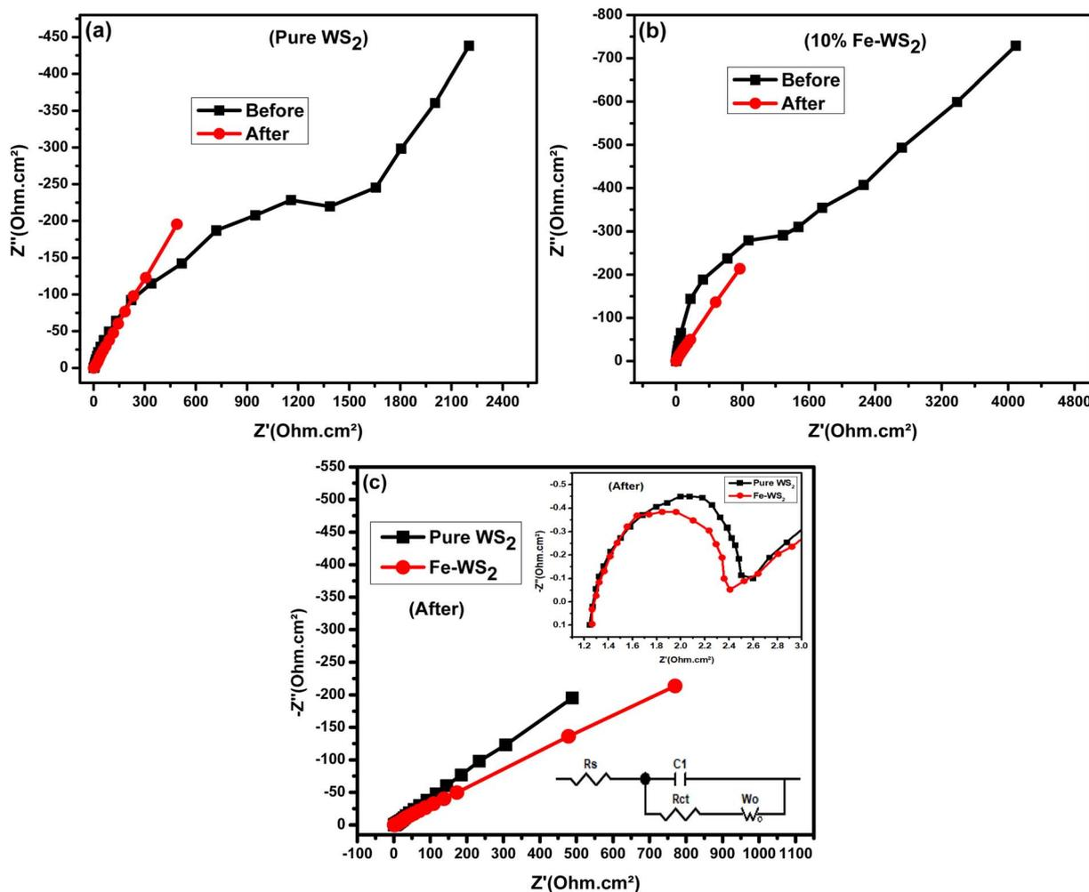
Fig. 10 (a) Nyquist plots before and after of pure WS<sub>2</sub>, (b) Nyquist plots before and after of Fe-WS<sub>2</sub> (c) Nyquist plots after GCD of pure and Fe-WS<sub>2</sub>.
