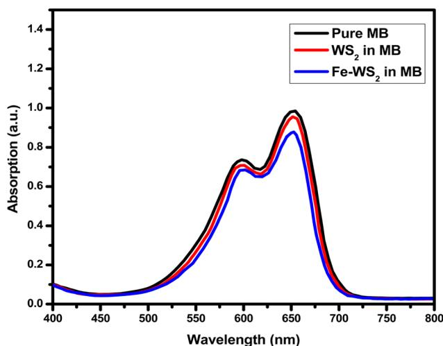
Fig. 7 UV absorption graph of pure WS<sub>2</sub> and Fe-doped WS<sub>2</sub> in MB.
