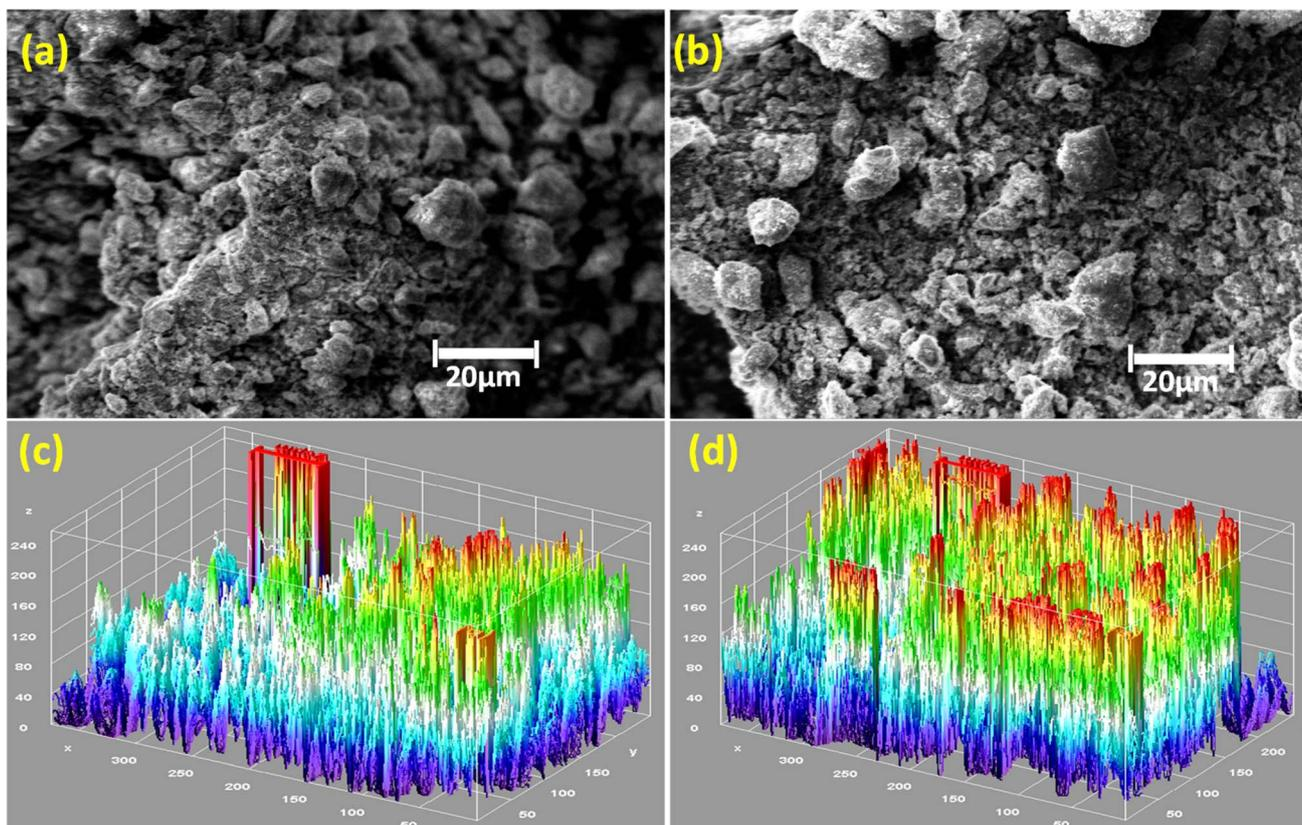
Fig. 5 (a) SEM image of pure WS<sub>2</sub> (b) SEM image of Fe-WS<sub>2</sub> (c) 3D image of pure WS<sub>2</sub> (d) 3D image of Fe-WS<sub>2</sub>.
