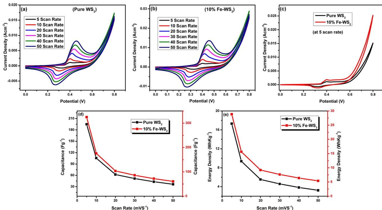
Fig. 8 (a) CV curves of pure electrode, (b) CV curves of doped electrode, (c) CV curves at 5 scan rate of both sample, (d) specific capacitance, (e) energy density of pure  $\text{WS}_2$  and  $\text{Fe-WS}_2$ .
