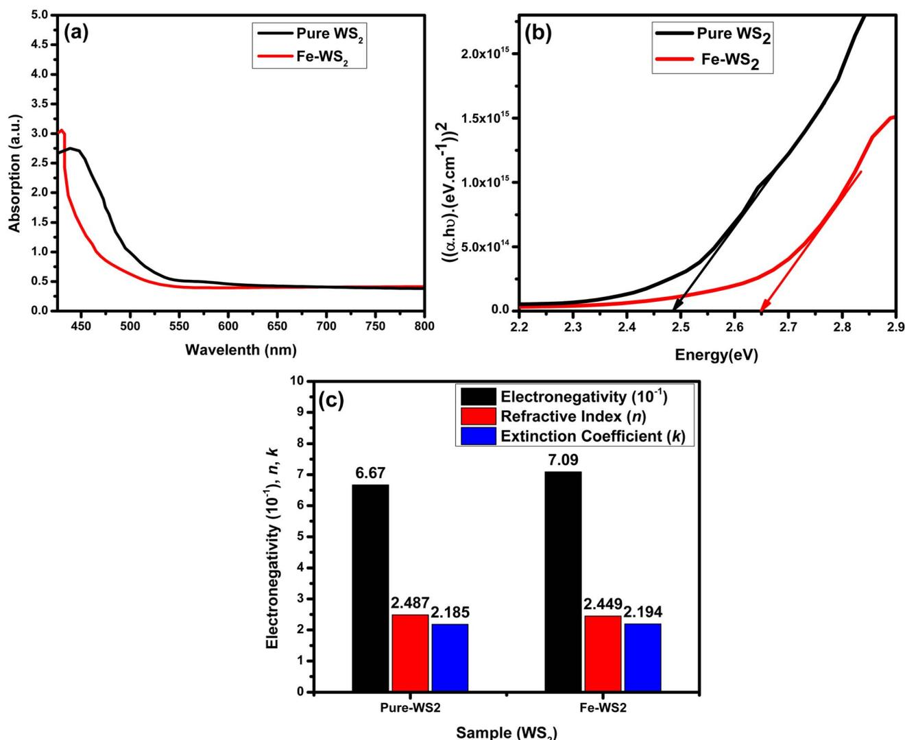
Fig. 6 (a) UV absorption graph, (b) Tau<sup>2</sup> graph, (c) graph between electronegativity refractive index and extinction coefficient of pure WS<sub>2</sub> and Fe-WS<sub>2</sub>.
