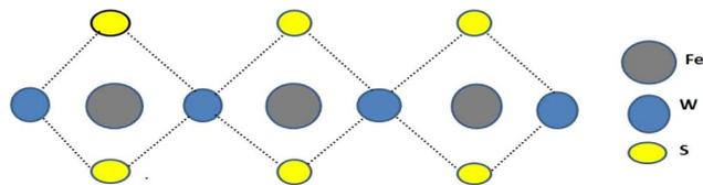
Fig. 1 Structure of Fe-WS<sub>2</sub> material.
