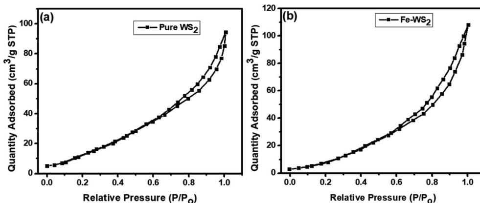
Fig. 4 BET analysis (a) pure WS<sub>2</sub> (b) Fe-doped WS<sub>2</sub> nanostructures.
