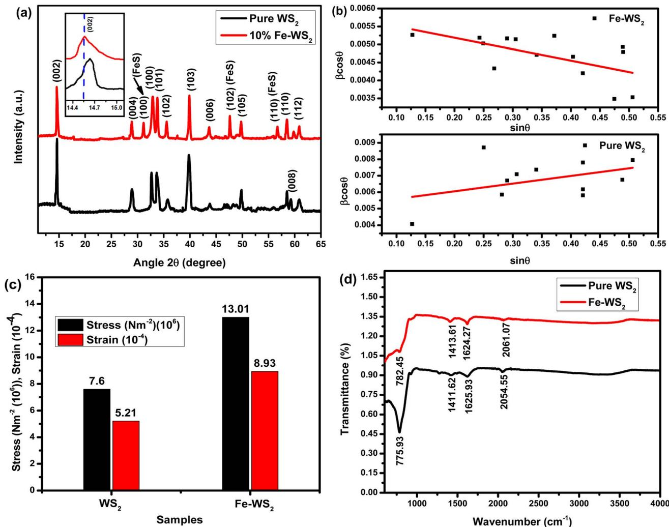
Fig. 3 (a) XRD pattern, (b) relation between grain size, dislocation line density and  $d$ -spacing, (c) relation between stress and strain, (d) FTIR graph of pure WS<sub>2</sub> and Fe-WS<sub>2</sub>.
