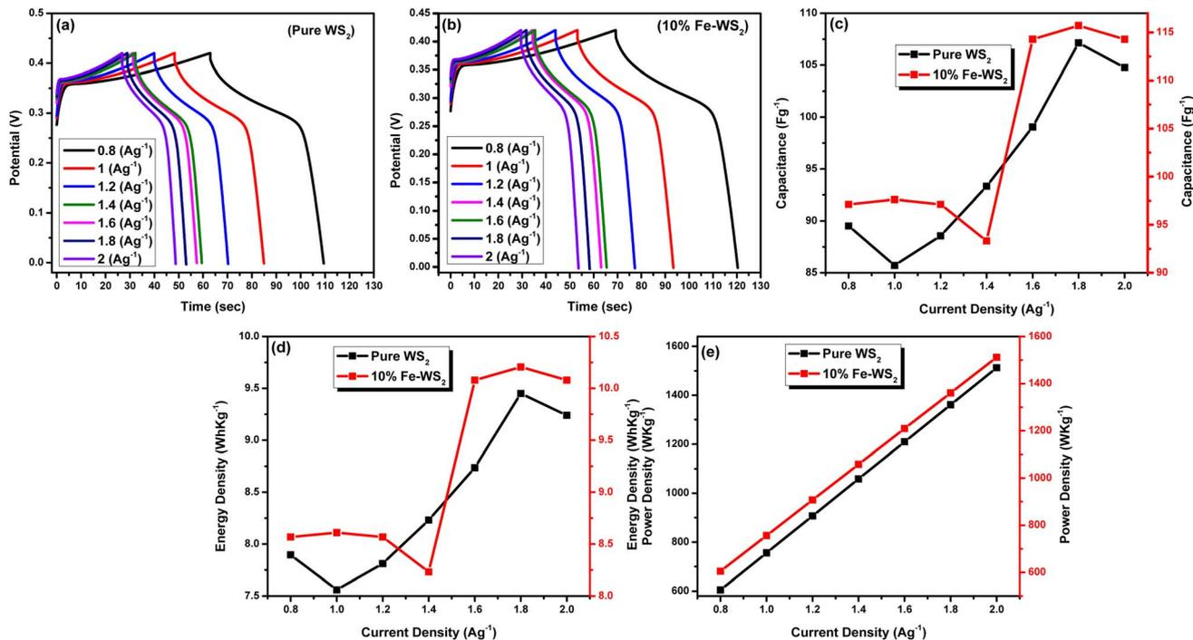
Fig. 9 (a) GCD curves of Pure WS<sub>2</sub> (b) GCD curves of Fe-WS<sub>2</sub> (c) capacitance of pure and Fe-doped sample (d) energy density of pure and Fe-doped sample (e) power density of pure and Fe-WS<sub>2</sub> sample.
