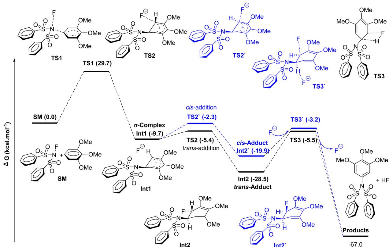
Fig. 1 Free energy profile for the amidation reaction at the wb97xd/6-311<sup>++</sup> level of theory.
