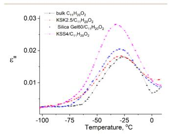
Fig. 2 Temperature dependencies of the imaginary part of dielectric permittivity of samples at  $f=50~\mathrm{kHz}$ .
