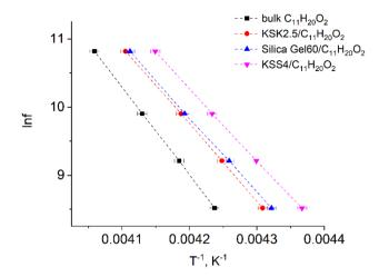
Fig. 3 Natural logarithm of electric field frequency vs. inverse temperature  $T_{\rm e}$  corresponding to the peak in the imaginary part of dielectric permittivity of samples.
