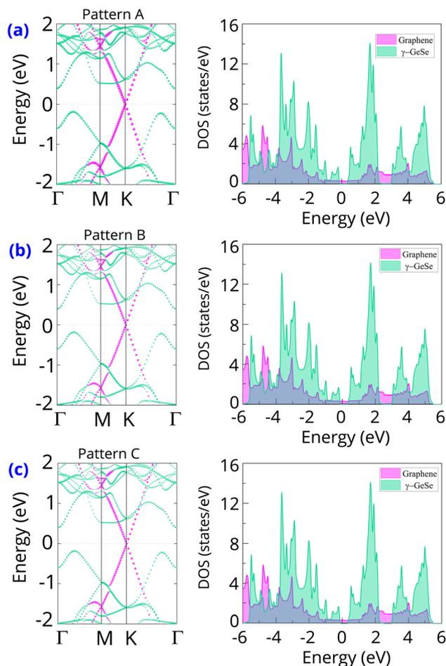
Fig. 3 The weighted projections in the band structures and density of states for each layer of the graphene/ $\gamma$ -GeSe heterostructure for the different patterns of (a) pattern A, (b) pattern B and (c) pattern C. Green and purple balls denote the weighted projections of the  $\gamma$ -GeSe and graphene layers, respectively.
