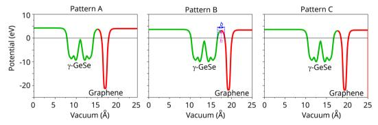
Fig. 5 Electrostatic potential of the graphene/ $\gamma$ -GeSe heterostructure for the different patterns.
