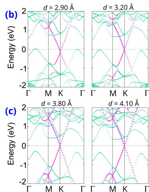
Fig. 7 (a) The evolution of the Schottky barriers in the graphene/ $\gamma$ -GeSe heterostructure under different interlayer spacings  $d$ . The projections of weighted bands of the graphene/ $\gamma$ -GeSe heterostructure with (b) decreasing and (c) increasing the interlayer spacings. Green and purple lines denote the projections of the  $\gamma$ -GeSe and graphene layers, respectively.
