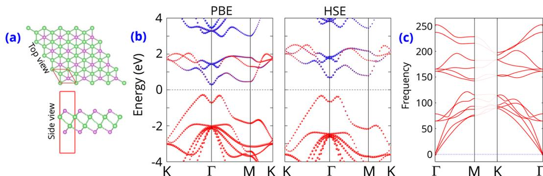
Fig. 1 (a) Atomic structure (b) band structures and (c) phonon spectra of  $\gamma$ -GeSe monolayer.
