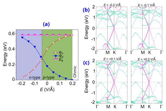
Fig. 6 (a) The evolution of the Schottky barriers in the graphene/ $\gamma$ -GeSe heterostructure under different values of electric fields. The projections of weighted bands of the graphene/y-GeSe heterostructure under the application of (b) negative and (c) positive values of electric field. Green and purple lines denote the projections of the  $\gamma$ -GeSe and graphene layers, respectively.
