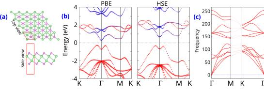
(a) Atomic structure (b) band structures and (c) phonon spectra of  $\gamma$ -GeSe monolayer
