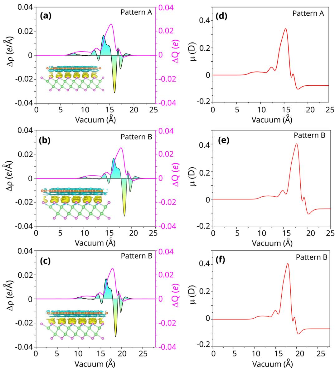
Fig. 4 Planar-average charge density difference and total amount of charge transfers of (a) pattern A, (b) pattern B and (c) pattern C. Interfacial dipole moment  $\mu$  of (d) pattern A, (e) pattern B and (f) pattern C of the graphene/ $\gamma$ -GeSe heterostructure. The charge accumulation (depletion) is denoted by the yellow (cyan) area.
