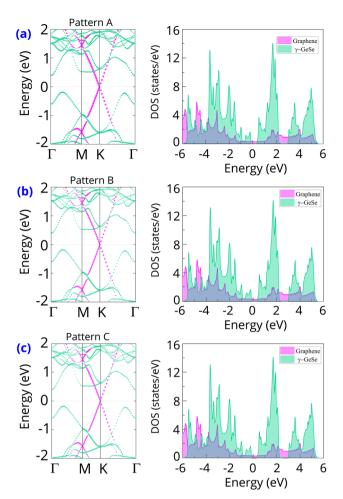
Fig. 3 The weighted projections in the band structures and density of states for each layer of the graphene/ $\gamma$ -GeSe heterostructure for the different patterns of (a) pattern A, (b) pattern B and (c) pattern C. Green and purple balls denote the weighted projections of the  $\gamma$ -GeSe and graphene layers, respectively.
