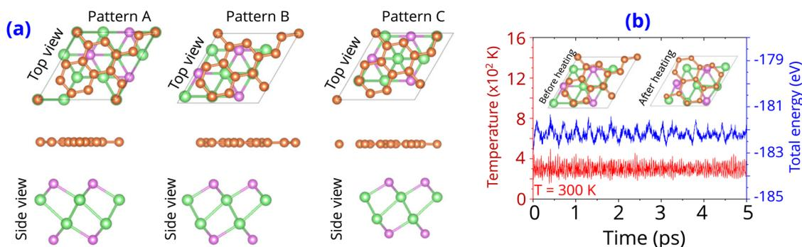
Fig. 2 (a) Atomic structures of the graphene/ $\gamma$ -GeSe heterostructure for different patterns. (b) AIMD simulation of the fluctuations in the total energy and temperature of the graphene/ $\gamma$ -GeSe heterostructure. The insets show the geometric structure the graphene/ $\gamma$ -GeSe heterostructure before and after the relaxation times up to 5 ps.
