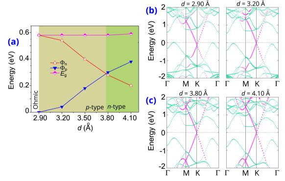
Fig. 7 (a) The evolution of the Schottky barriers in the graphene/ $\gamma$ -GeSe heterostructure under different interlayer spacings d. The projections of weighted bands of the graphene/γ-GeSe heterostructure with (b) decreasing and (c) increasing the interlayer spacings. Green and purple lines denote the projections of the  $\gamma$ -GeSe and graphene layers, respectively.
