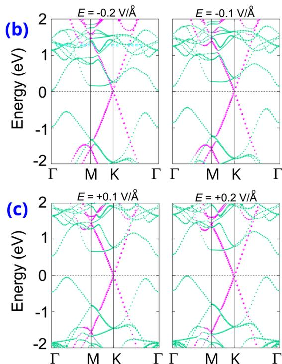
Fig. 6 (a) The evolution of the Schottky barriers in the graphene/ $\gamma$ -GeSe heterostructure under different values of electric fields. The projections of weighted bands of the graphene/ $\gamma$ -GeSe heterostructure under the application of (b) negative and (c) positive values of electric field. Green and purple lines denote the projections of the  $\gamma$ -GeSe and graphene layers, respectively.
