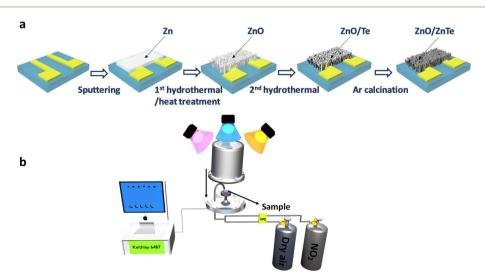
Fig. 1 (a) Fabrication process of ZnO/ZnTe nanohybrid structures and (b) schematic of the gas detection system.
