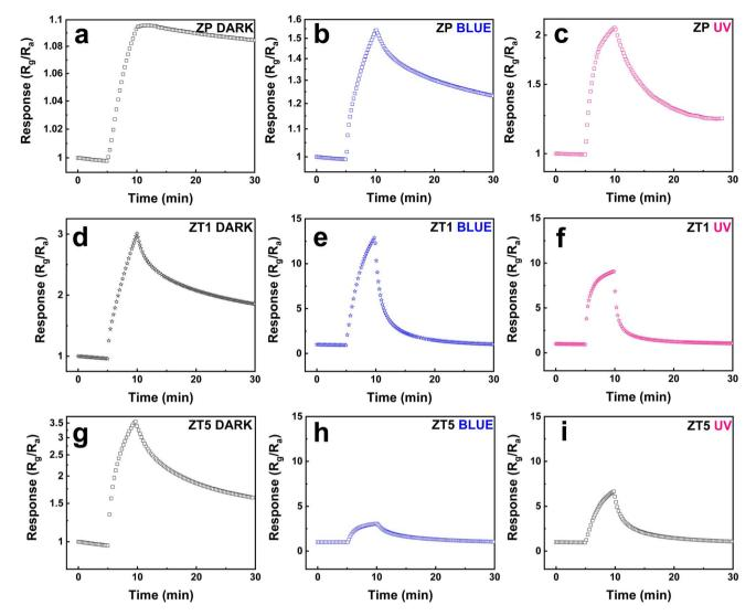
Response curves to 500 ppb NO<sub>2</sub> of (a-c) ZP, (d-f) ZT1, (g-i) ZT5 under dark, blue, and UV irradiation sources
