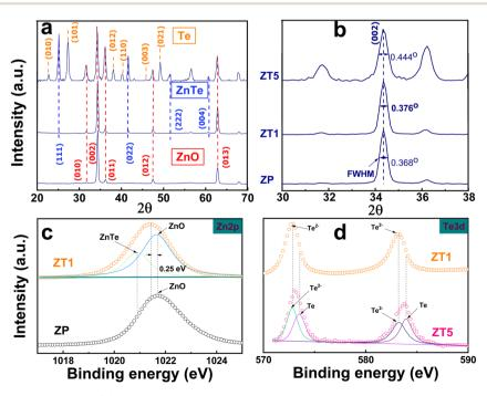
Fig. 2 (a) XRD pattern of ZP, ZT1, and ZT5. (b) The full width at half maximum (FWHM) for three samples. The XPS profiles for (c) Zn 2p of ZP compared with ZT1, and (d) Te 3d from ZT1 and ZT5.
