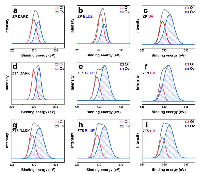
ig. 4 Deconvoluted O 1s XPS core-level spectra of (a-c) ZP; (d-f) ZT1; (g-i) ZT5 under dark, blue, and UV light illumination effect.
