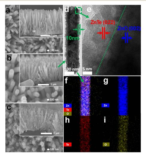
Fig. 3 Plan-view SEM illustration and cross-section images (inset) of (a) ZP, (b) ZT1, and (c) ZT5 samples. (d and e) TEM profiles of ZT1 and (f–i) elemental mapping images of ZT1.
