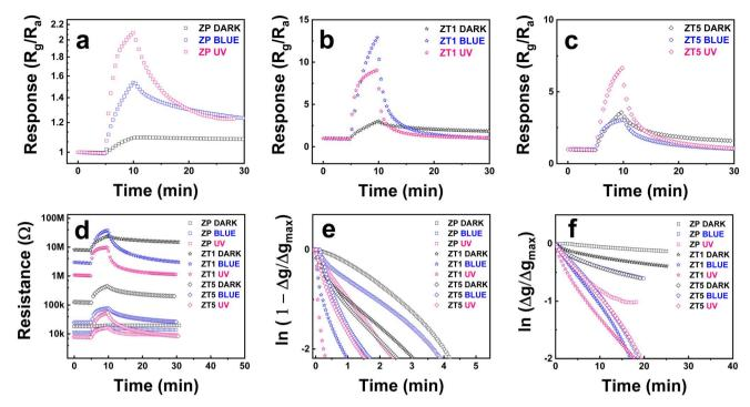
Fig. 6 (a–c) The response curves, (d) the resistance behaviors, the plots of (e) the response time, and (f) the recovery time of ZP, ZT1, and ZT5 toward 500 ppb  $NO_2$  exposal at different light irradiation situations.
