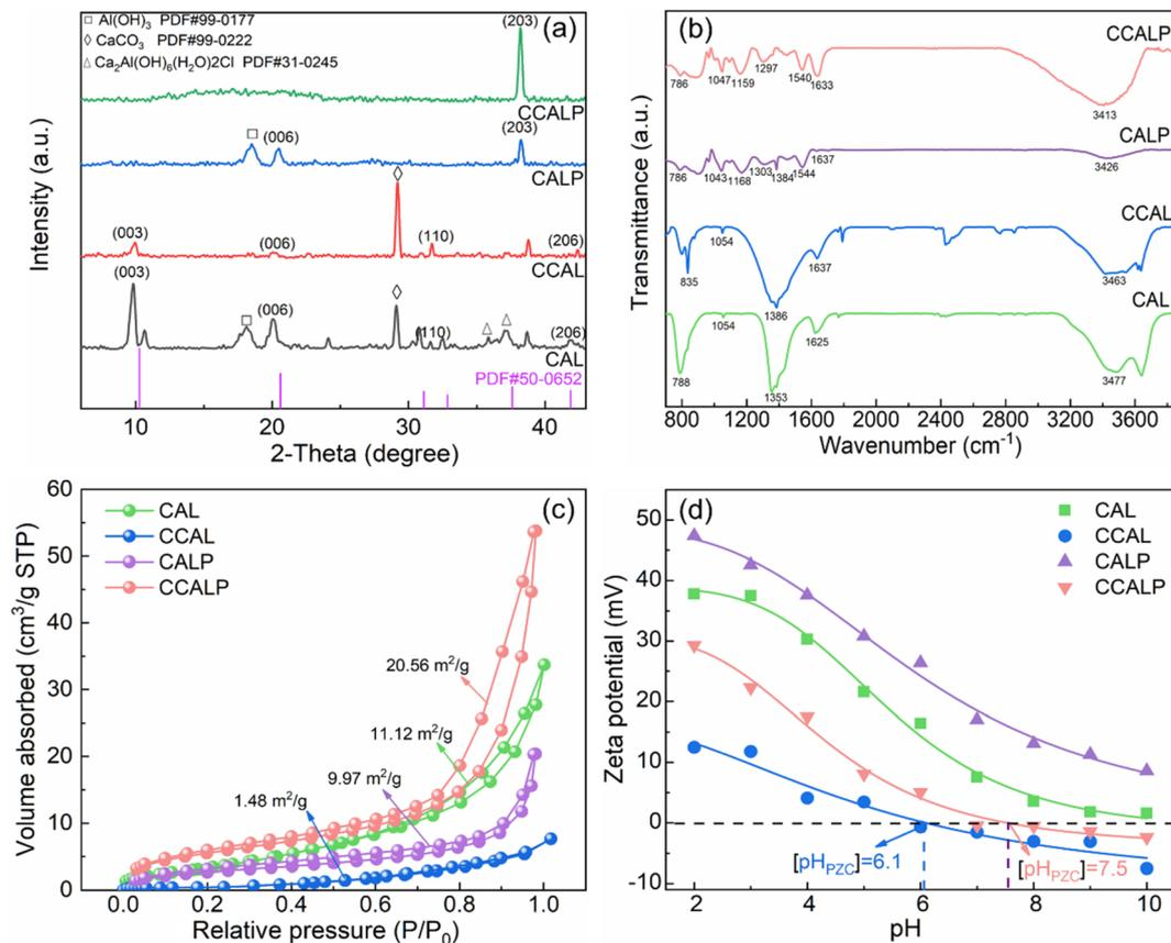
Fig. 2 (a) XRD patterns, (b) ATR-FTIR spectra, (c) N<sub>2</sub> adsorption–desorption isotherms (d) zeta potential, of CAL, CCAL, CALP and CCALP.
