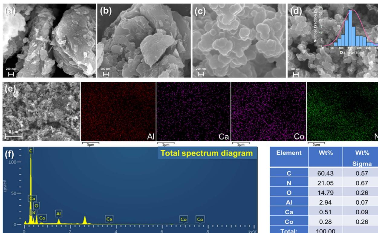
Fig. 1 SEM images of (a) CAL, (b) CCAL, (c) CALP and (d) CCALP. (e) EDS mapping of Al, Ca, Co and N in CCALP. (f) Total spectrum and table of element content of the CCALP.
