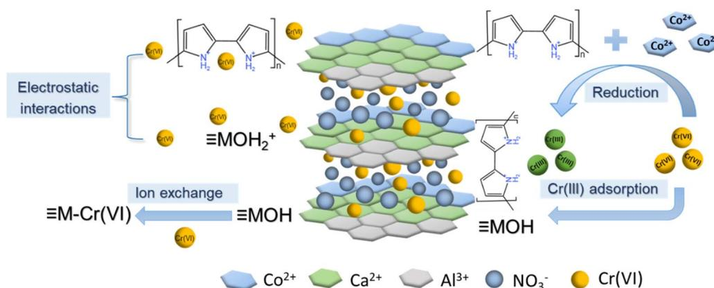
Fig. 11 Proposed adsorption mechanism of Cr(VI) on CCALP.
