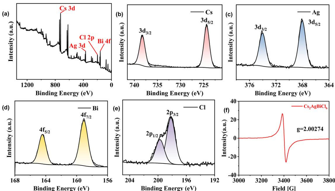
Fig. 4 (a) XPS full spectrum of  $\text{Cs}_2\text{AgBiCl}_6$ -DP SCs; XPS characterization of Cs 3d (b), Ag 3d (c), Bi 4f (d) and Cl 2p (e) in  $\text{Cs}_2\text{AgBiCl}_6$ -DP SCs; (f) EPR curve of  $\text{Cs}_2\text{AgBiCl}_6$ -DP SCs.
