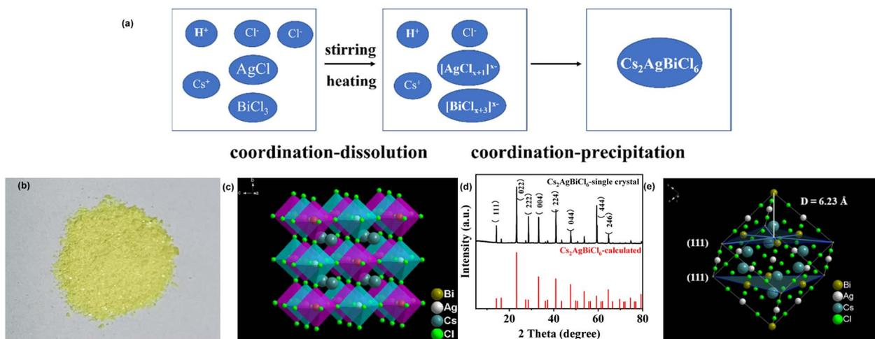
Fig. 1 (a) Schematic of coordination-dissolution and coordination-precipitation reaction; (b) photograph of  $\text{Cs}_2\text{AgBiCl}_6$  crystal powder; (c) three-dimensional crystal structure of  $\text{Cs}_2\text{AgBiCl}_6$ -DP SCs determined by single crystal X-ray diffraction results; (d) XRD patterns of  $\text{Cs}_2\text{AgBiCl}_6$ -DP SCs obtained by PXRD and calculated by single crystal information data with Diamond software; (e) schematic of interplanar spacing of (111) crystal plane.
