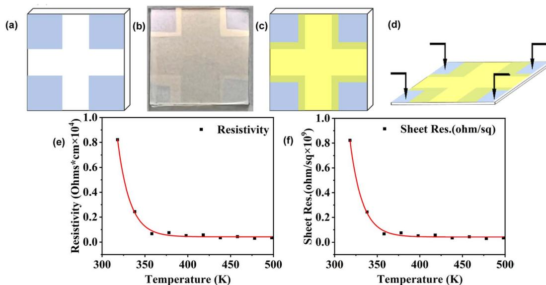
Fig. 7 Resistance characteristics of  $\text{Cs}_2\text{AgBiCl}_6$  DP thin film: (a) schematic of conductive glass substrate layout (four blue squares represent conductive areas); (b) photograph of the evaporated  $\text{Cs}_2\text{AgBiCl}_6$  DP thin film on conductive glass; (c) schematic of (b); (d) schematic of four-probe testing; (e) curve of resistivity variation with temperature; (f) curve of square resistance variation with temperature.
