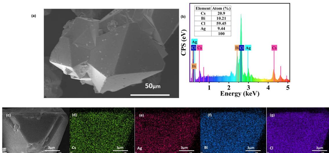
Fig. 2 (a) SEM image of Cs<sub>2</sub>AgBiCl<sub>6</sub>-DP SCs; (b) EDS spectrum and element content of Cs<sub>2</sub>AgBiCl<sub>6</sub>-DP SCs; (c) the region corresponding to element mapping of Cs (d), Ag (e), Bi (f) and Cl (g) in Cs<sub>2</sub>AgBiCl<sub>6</sub>-DP SCs.
