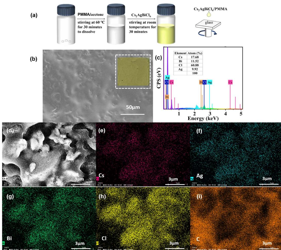
Fig. 5 (a) Preparation process of  $\text{Cs}_2\text{AgBiCl}_6$ -DP thin film on glass; (b) SEM image of surface morphology of  $\text{Cs}_2\text{AgBiCl}_6$ -DP particles in  $\text{Cs}_2\text{AgBiCl}_6$ -DP thin film; (c) EDS spectrum and content of  $\text{Cs}_2\text{AgBiCl}_6$ -DP thin film; (d) the region corresponding to element mapping of Cs (e), Ag (f), Bi (g), Cl (h) and C (i) in  $\text{Cs}_2\text{AgBiCl}_6$ -DP thin film.
