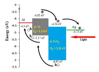
Fig. 20 Illuminated energy band diagram of FeS<sub>2</sub>/p-Si heterojunction under reverse bias.
