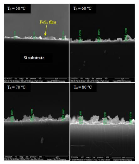
Fig. 4 SEM images cross section of FeS<sub>2</sub> films deposited on silicon substrates at various temperatures.
