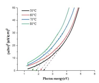
Fig. 7 Plot of  $(\alpha hv)^2$  versus photon energy of FeS<sub>2</sub> films deposited at different temperature using laser.
