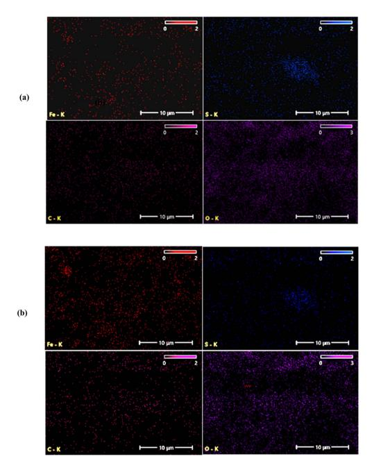
Fig. 10 EDX mapping of FeS<sub>2</sub> film deposited at (a)  $T_d = 50$  °C and (b)  $T_d = 60$  °C.
