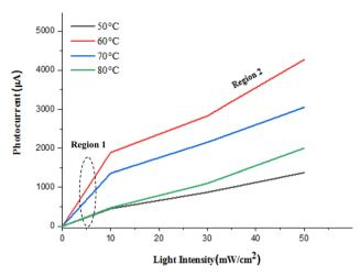
Fig. 16 Variation of photocurrent with light intensity of n-FeS<sub>2</sub>/p-Si photodetectors deposited at different temperatures.
