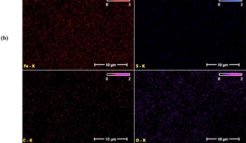
Fig. 11 EDX mapping of FeS<sub>2</sub> film deposited at (a)  $T_d = 70$  °C and (b)  $T_d = 80$  °C.
