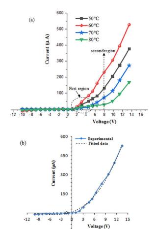
Fig. 14 (a) Dark I-V characteristics of n-FeS<sub>2</sub>/p-Si heterojunctions prepared at various deposition temperatures and (b) experimental and fitted I-V curves for heterojunction deposited at  $T_{\rm d}=60$  °C.
