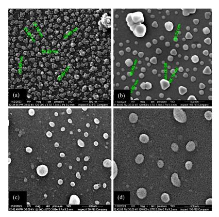
Fig. 8 SEM images of FeS<sub>2</sub> films deposited at (a) 50, (b) 60, (c) 70, and (d) 80 °C.
