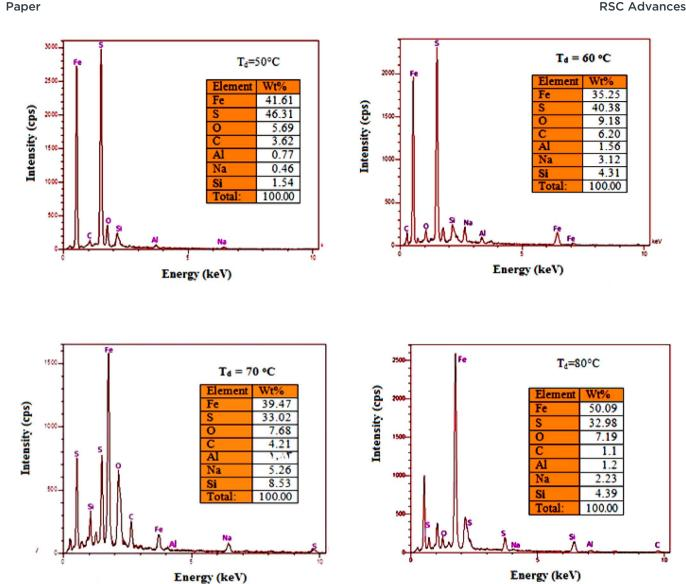
EDX spectra of FeS<sub>2</sub> films deposited at different temperatures. Inset is the weight percentage of the elements in FeS<sub>2</sub> film.
