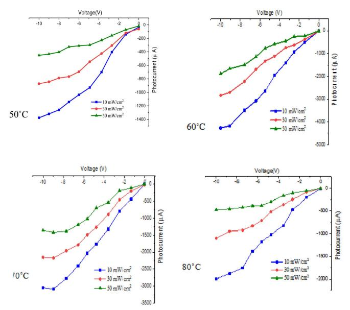
Fig. 15 Illuminated I-V characteristics of n-FeS<sub>2</sub>/p-Si heterojunctions deposited at different temperatures
