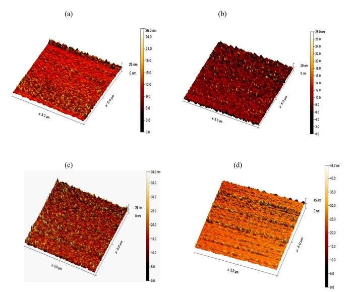
Fig. 12 3-D AFM images of FeS<sub>2</sub> films deposited at various temperatures (a) 50 °C, (b) 60 °C, (c) 70 °C, and (d) 80 °C.
