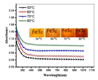
Fig. 6 Effect of deposition temperature on the optical absorbance of FeS<sub>2</sub> film. Inset is the photographs of films deposited at various deposition temperatures.
