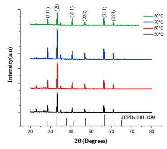
Fig. 5 XRD patterns of FeS<sub>2</sub> films grown at different temperatures.
