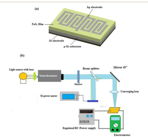
Fig. 2 (a) Cross section view of FeS<sub>2</sub>/Si photodetector and (b) schematic diagram of cross-sectional view of the Aq-FeS<sub>2</sub>/n-Si-Al photodetector.
