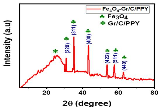
Fig. 4 XRD exploration of multi-layered  $\text{Fe}_3\text{O}_4$ -Gr/C/PPy nanofiber composite.
