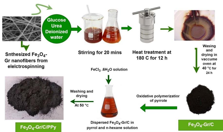
Fig. 1 Pictorial representation of synthesis processes of Fe<sub>3</sub>O<sub>4</sub>-Gr/C/PPy nanofibers composite.
