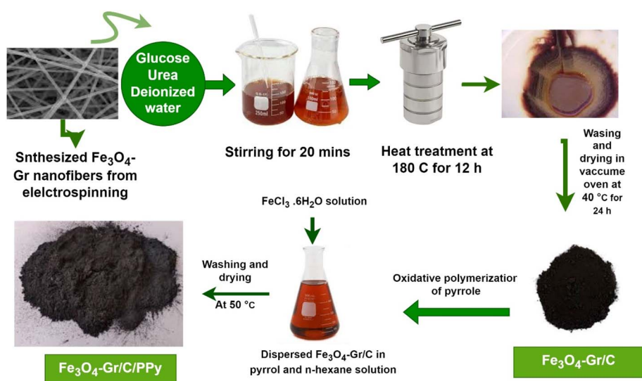
Fig. 1 Pictorial representation of synthesis processes of Fe 3 O 4 -Gr/C/PPy nanofibers composite.
