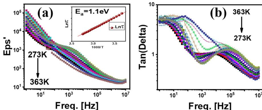
Fig. 7 (a) The dielectric constant and (b) tangent loss analysis of the Fe<sub>3</sub>O<sub>4</sub>-Gr/C/PPy nanofiber composite.
