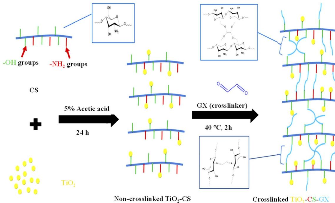
Fig. 4 Synthesis of  $\text{TiO}_2$ -CS-GX by simultaneously mixing  $\text{TiO}_2$ , CS followed by GX crosslinkers (reproduced from ref. 125 with permission from Elsevier, copyright 2019).<sup>125</sup>
