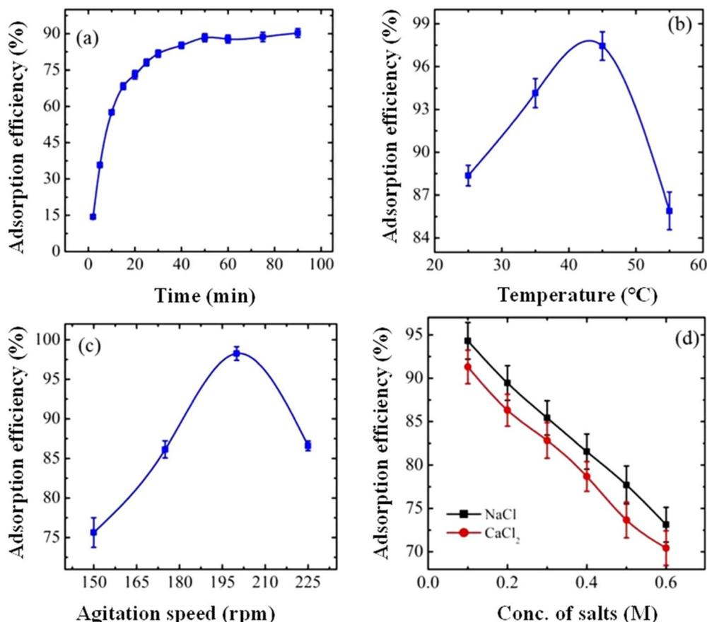
Fig. 9 Effect of parameters on the adsorption of pollutants: (a) contact time, (b) temperature, (c) agitation speed, and (d) salt concentrations (reproduced from ref. 132 with permission from Elsevier, copyright 2016).<sup>132</sup>
