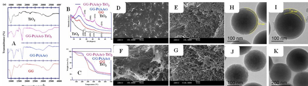
Fig. 5 Characterization techniques: (A) FTIR, (B) XRD and (C) TGA (reproduced from ref. 71 and 102 with permission from Elsevier, copyright 2022).<sup>71,102</sup> (D–G) SEM image (reproduced from ref. 74 with permission from Elsevier, copyright 2021).<sup>74</sup> (H–K) TEM image (reproduced from ref. 95 with permission from Elsevier, copyright 2019).<sup>95</sup>
