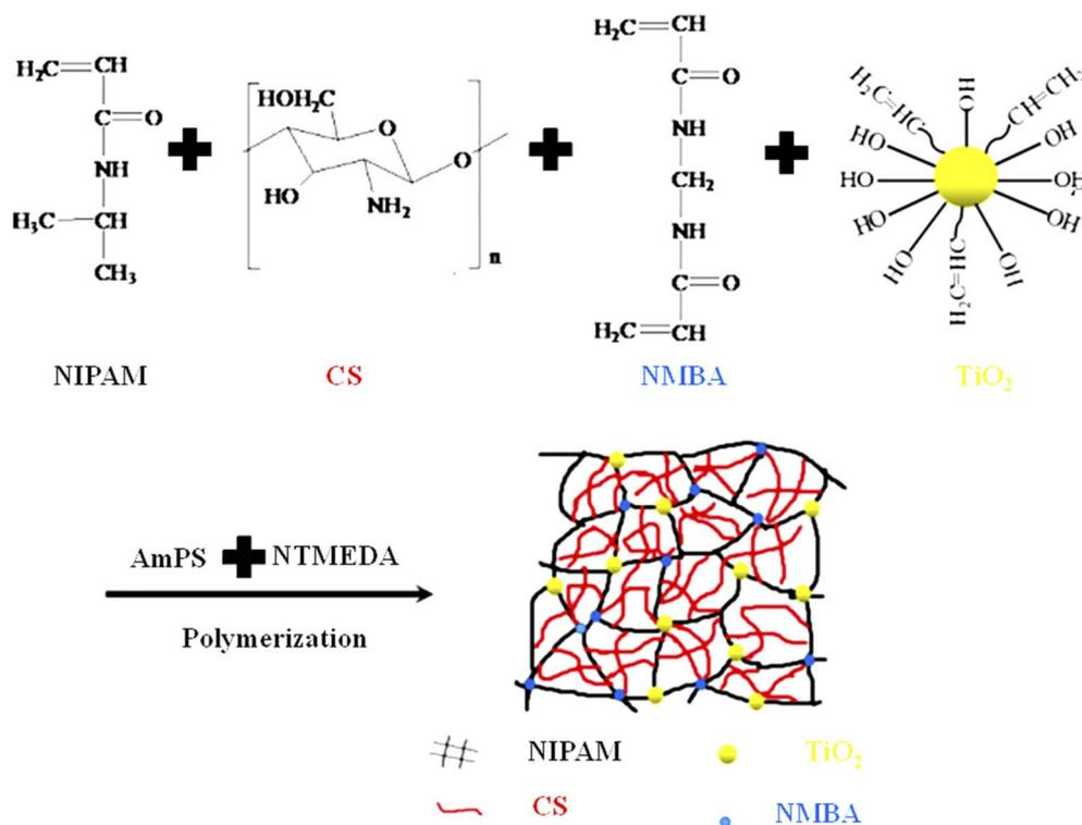
Fig. 2 Synthesis of  $\text{TiO}_2$  nanoparticles decorated in chitosan-poly(*N*-isopropylacrylamide) ( $\text{TiO}_2$ -CS-P(NIPAM)) by simultaneously mixing all components (reproduced from ref. 102 with permission from Elsevier, copyright 2017).<sup>102</sup>
