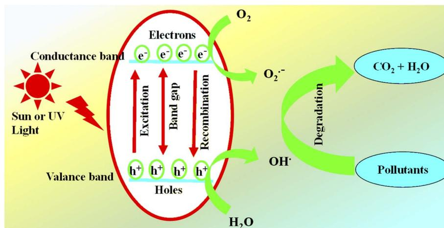
Fig. 10 Photocatalytic degradation mechanism.
