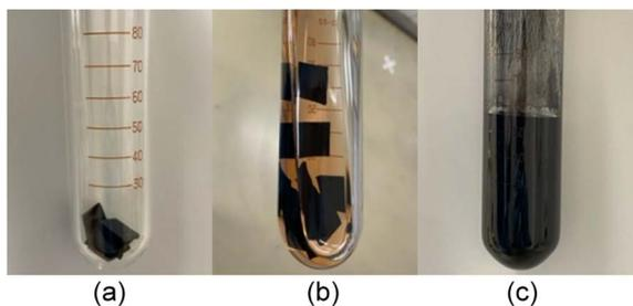
Fig. 5 Photos of crosslinked poly(CP) rubber in an ampoule tube (a), just after adding G2 solution (b) and 24 h after the depolymerization reaction at 60 °C (c).
