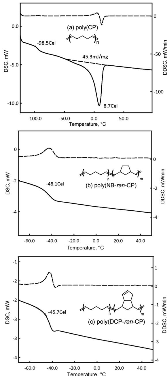
Fig. 2 DSC charts of (a) poly(CP), (b) poly(NB-ran-CP) and (c) poly(DCP-ran-CP) (determined in the second scan under N<sub>2</sub> for 10 °C min<sup>-1</sup> after full annealing; solid line is DSC; dashed line is DDSC).
