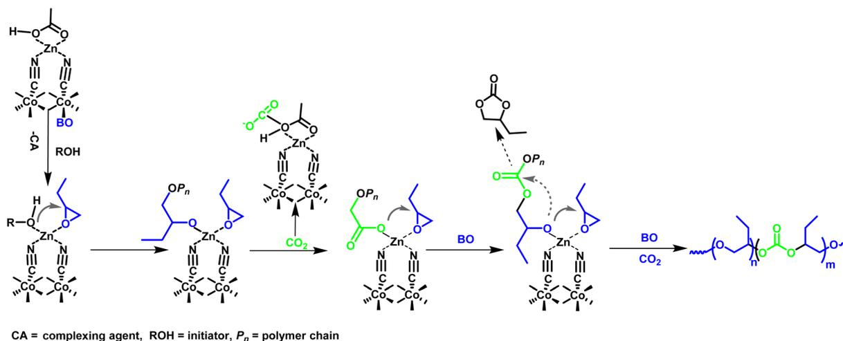
Scheme 2 Proposed mechanism for the copolymerization of CO<sub>2</sub> and BO using L-DMC catalyst.
