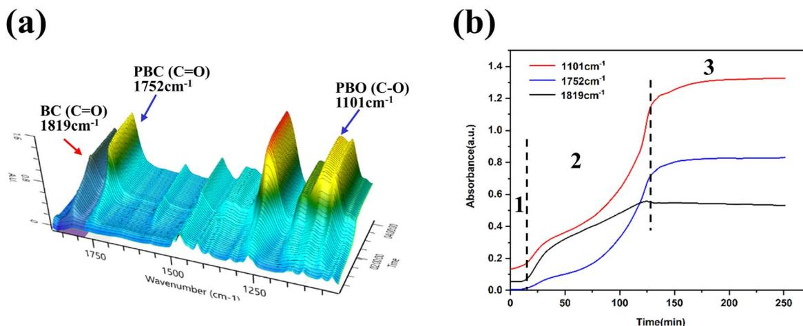
Fig. 4 (a) Three-dimensional stack plots of *in situ* FTIR spectroscopy. (b) Reaction profile monitored by *in situ* FTIR. Reaction was carried out at 110 °C, 1.5 MPa CO<sub>2</sub> pressure.
