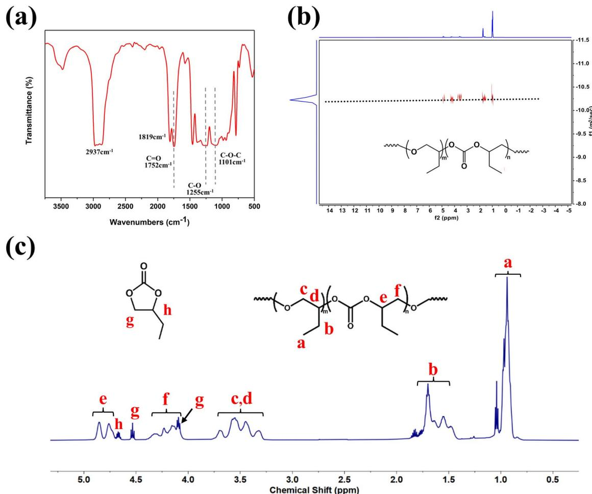
Fig. 5 Preparation of the polycarbonate ether polyol (Table 1, entry 2) by the copolymerization of CO<sub>2</sub> and BO using L-DMC. (a) FTIR spectrum. (b) DOSY NMR spectrum. (c) <sup>1</sup>H-NMR spectrum.
