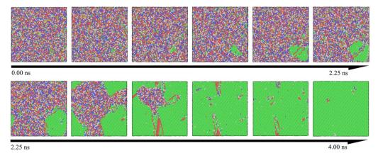
Fig. 4 Snapshots of the crystallization process in the Ni-Fe alloy model are presented, with atoms of different structures assigned distinct colors: FCC is shown in green, BCC in blue, and HCP in red, while other colors represent atoms that have not yet formed a lattice structure. The snapshots illustrate the dynamic evolution during crystallization, revealing the appearance of nuclei, the growth of crystals, and transitions between different structures over time and temperature.
