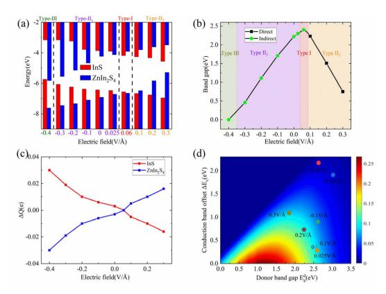
Fig. 4 The band alignments (a), band gaps (b), and charge transfer (c) of the InS/ZnIn<sub>2</sub>S<sub>4</sub> heterostructure under different electric fields. (d) The  $\eta$  of the InS/ZnIn<sub>2</sub>S<sub>4</sub> heterostructure as a function of  $\Delta E_c$  and  $E_c^d$  under different electric fields.
