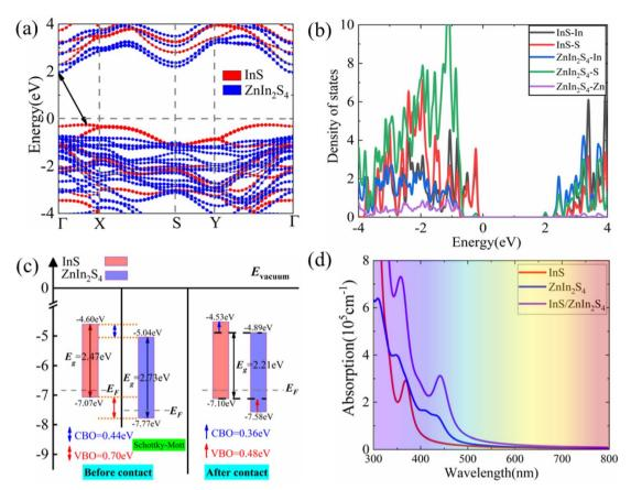
Fig. 3 The projected band structure (a), projected DOS (b), band alignment (c), and absorption spectra (d) of the InS/ZnIn<sub>2</sub>S<sub>4</sub> heterostructure using the vacuum energy levels as a common energy reference.  $E_q$  and  $E_F$  denote the energies of the bandgap and Fermi energy levels, respectively. The CBO and VBO are represented by blue and red arrows, respectively.
