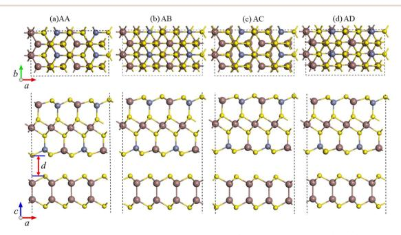
Fig. 1 Top and side views of the four possible stacking configurations of the  $InS/ZnIn_2S_4$  heterostructures: (a) AA, (b) AB, (c) AC, and (d) AD. d represents the interlayer distance.
