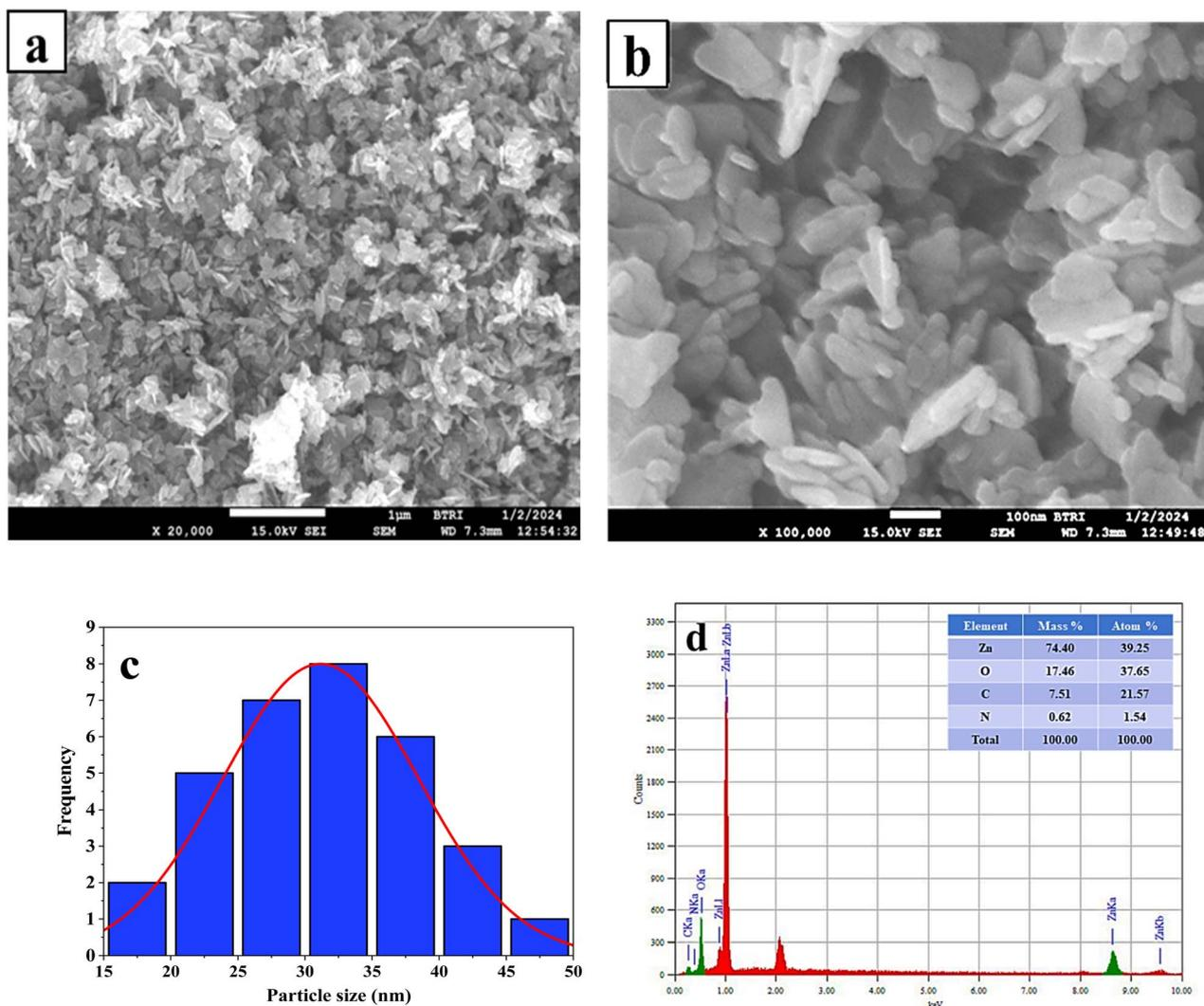
Fig. 4 (a) and (b) FE-SEM micrograph of ZPCL synthesized from *C. lanatus* rind extract, (c) histogram of particle size of ZPCL, and (d) EDX spectrograph of ZPCL.
