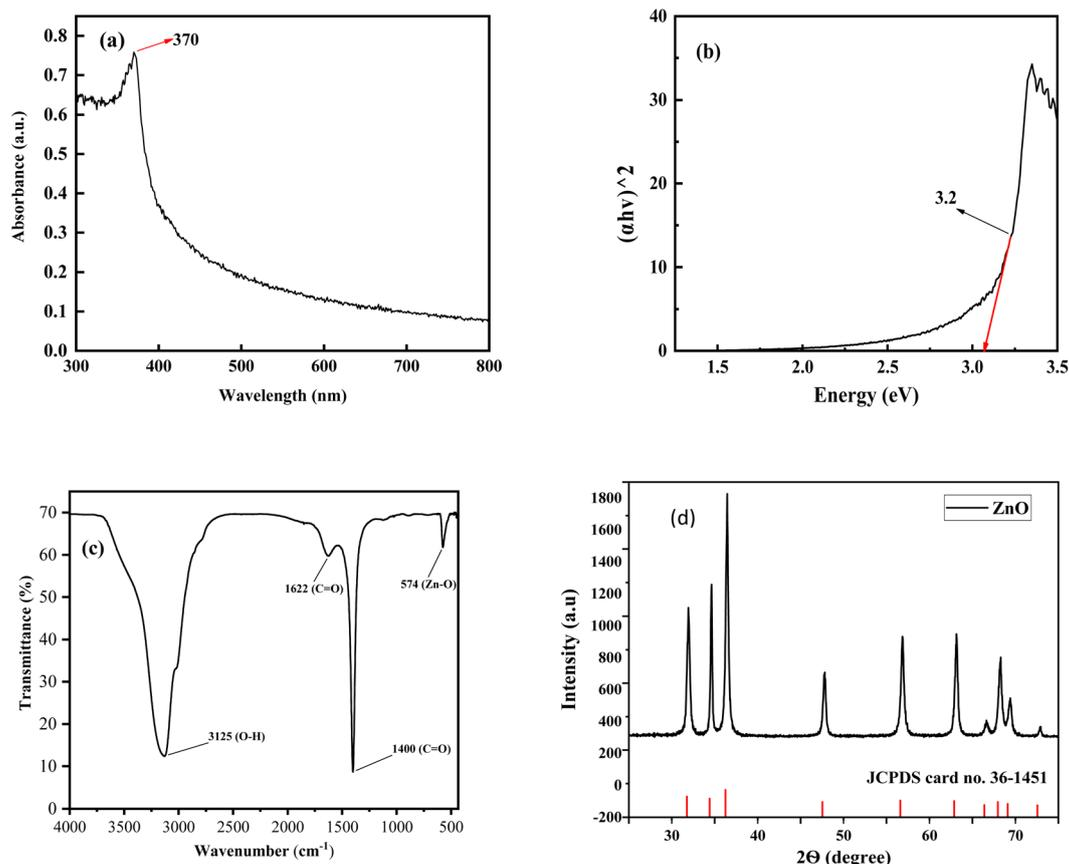
Fig. 3 (a) UV-vis spectrum of ZPCL synthesized using *C. lanatus* rind extract, (b)  $(\alpha h\nu)^2$  versus the photon energy ( $h\nu$ ) for ZPCL, (c) FT-IR spectra of nanocrystalline ZPCL, (d) XRD pattern of the produced ZPCL (the bottom bars show the standard ZnO from JCPDS No. 36-1451).
