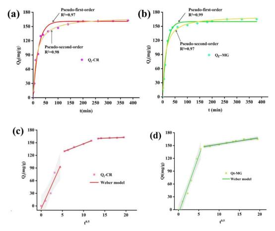
Fig. 8 (a and b) Pseudo-first-order kinetics and pseudo-second-order kinetics plots CR and MG adsorption on composite fibers; (c and d) Weber–Morris model kinetics plots CR and MG adsorption on composite fibers.
