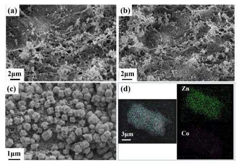
Fig. 2 SEM images of ZIF-8@CS (a), ZIF-67@CS (b) and Zn-Co-ZIF@CS (c), and SEM mapping images of Zn-Co-ZIF@CS (d).
