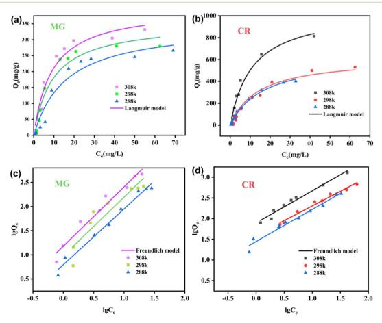
Fig. 9 (a and b) Fitting of the Langmuir model for adsorption isothermal plots of ZIF-8@CS toward MG and CR; (c and d) Freundlich model for adsorption isothermal plots of ZIF-8@CS toward MG and CR.
