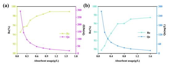
Fig. 5 Removal efficiency curves of CR (a) and MG (b) dyes with different adsorbent ZIF-8@CS dosages ( $R_e$ : removal efficiency;  $Q_e$ : adsorption capacity).
