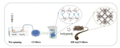
Fig. 1 Schematic illustration of the preparation of ZIF-n@CS composite fibers.
