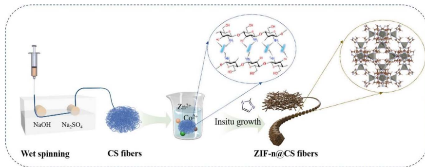
Fig. 1 Schematic illustration of the preparation of ZIF- n @CS composite fibers.
