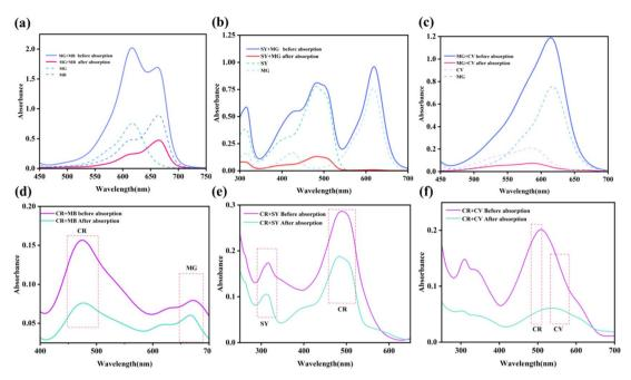
Fig. 7 UV-vis curves before and after the adsorption process in a binary mixed dye solution system (a) MG + MB system; (b) SY + MG system; (c) MG + CV system; (d) CR + MB system (e) CR + SY system; (f) CR + CV system.
