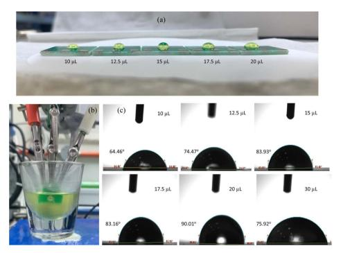
Fig. 6 (a) shows the PCB-3T loaded with variable microdroplet volumes, (b) PCB-3T sensor immersed in 10 mL of  $K_3$ [Fe(CN)<sub>6</sub>] solution and (c) droplet contact angle measurements of PCB-3T sensor performed on Biolin Scientific Attension Theta Lite Optical Tensiometer.
