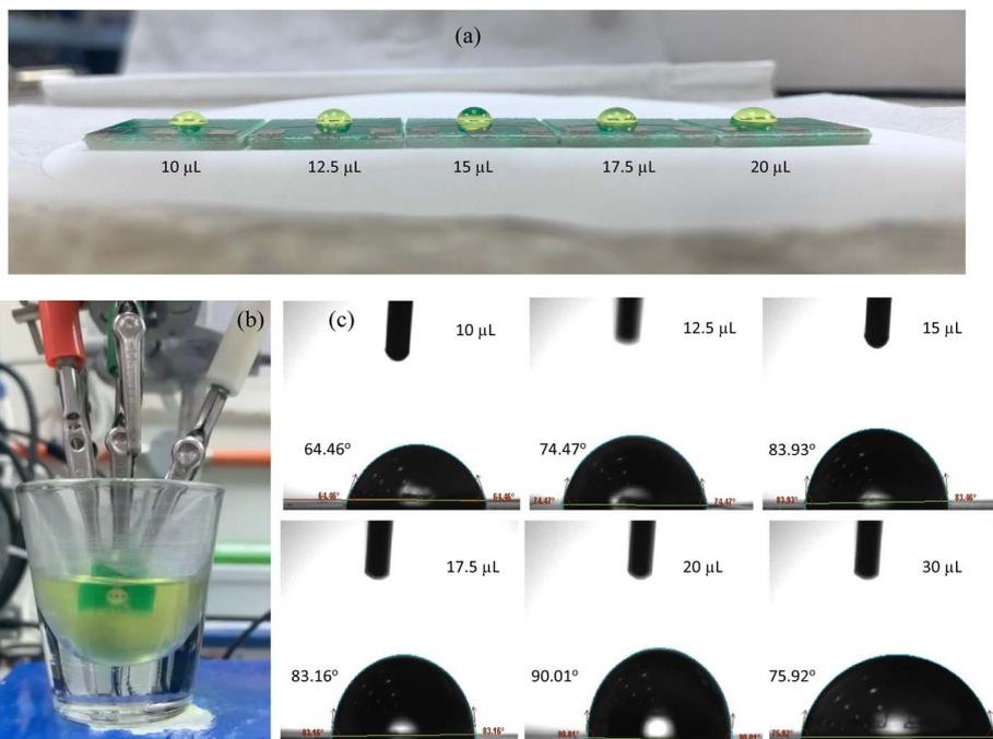
Fig. 6 (a) shows the PCB-3T loaded with variable microdroplet volumes, (b) PCB-3T sensor immersed in 10 mL of  $K_3[Fe(CN)_6]$  solution and (c) droplet contact angle measurements of PCB-3T sensor performed on Biolin Scientific Attension Theta Lite Optical Tensiometer.
