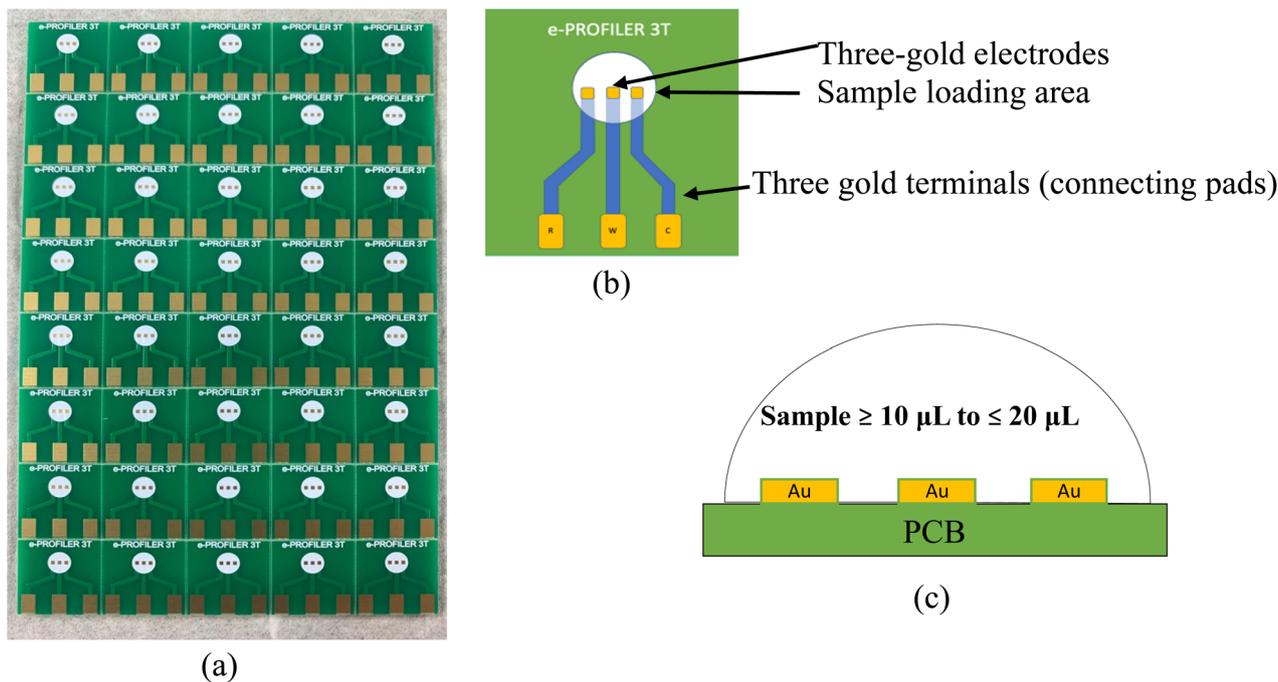
Fig. 1 Image showing the (a) proprietary PCB-3T electrode array on a  $120 \times 75$  mm PCB board, (b) schematic top view of PCB-3T sensor and (c) schematic lateral view of PCB-3T loading area.
