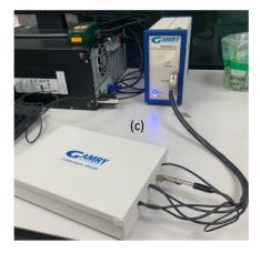
Fig. 3 Image shows photograph of (a) PCB-3T connected in RWC configuration, (b) shows the Gamry Reference 600 potentiostat connected to the sensor, (c) shows the Faraday cage enclosure used during experimentation.
