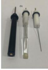
Fig. 2 Image shows photograph of (a) gold disk working electrode, Ag/AgCl reference electrode and platinum wire electrode in a conventional experimental setup with larger volume 10 mL of potassium ferricyanide solution in a glass vial. Figure (b) meanwhile shows the cross-sectional image of the gold disk working electrode, Ag/AgCl reference electrode and the platinum wire counter electrodes.
