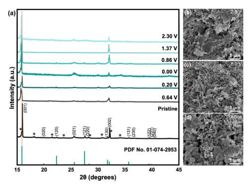
Fig. 5 (a) XRD spectra of VO- $H_3O$  from pristine state to various states of cycling: discharged from 2.30 to 0.0 V and charged from 0.0 to 2.3 V, and reference spectra (PDF No. 01-074-2953). SEM images of cathode material in (b) pristine state, (c) fully charged state to 2.3 V, and (d) fully discharged state to 0.0 V.
