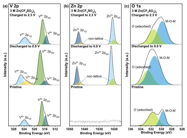
Fig. 6 XPS analysis of (a) V 2p, (b) Zn 2p, and (c) O 1s orbitals for VO-H<sub>3</sub>O cathode material with 3 M Zn(CF<sub>3</sub>SO<sub>3</sub>)<sub>2</sub> electrolyte at different states of cycling.
