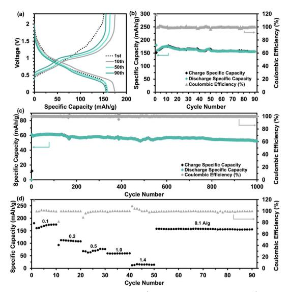
Fig. 4 (a) GCD profile, (b) corresponding cycling performance at  $0.1\,\mathrm{A\,g^{-1}}$ , (c) long-term cycling performance at  $1\,\mathrm{A\,g^{-1}}$ , and (d) rate performance at a current density range of 0.1 to  $1.4\,\mathrm{A\,g^{-1}}$  of VO-H<sub>3</sub>O cathode material in coin cells against  $\mathrm{Zn/Zn^{2+}}$  with 3 M  $\mathrm{Zn(CF_3SO_3)_2}$  as aqueous electrolyte.
