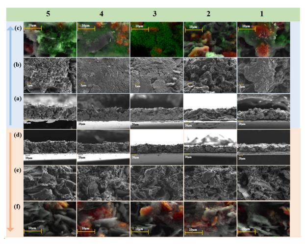
Fig. 7 SEM images and mapping results of Si/C pole pieces with different Si/C loadings for Samples 5–1. After 100 charge-discharge cycles: (a) SEM images of the cross-section. (b) SEM images of the surface. (c) Si (red) and O (green) mapping results for the surface. Fresh (d) SEM images of the cross-section. (e) SEM images of the surface. (f) Si (red) and O (green) mapping results for the surface.
