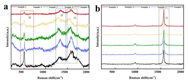
Fig. 6 Raman patterns of Si/C pole pieces with different Si/C loadings: (a) fresh and (b) after 100 cycles.
