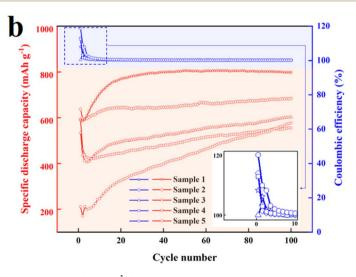
Fig. 1 Electrochemical performance of battery cells with different Si/C loadings at 300 mA  $\rm g^{-1}$ : (a) initial charge—discharge curves and (b) cycling stability.
