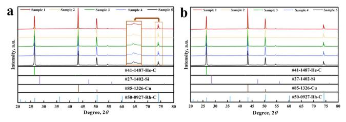
Fig. 5 XRD patterns of Si/C pole pieces with different Si/C loadings: (a) fresh and (b) after 100 cycles.
