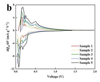
Standardized differential capacity curves ( $dQ_m/dV$  curves): (a) initial and (b) for the 100th charge-discharge cycle
