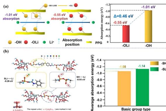
Fig. 7 (a) Effect of the functional group "-OH" on the adsorption energy of ions in the system; (b) change of adsorption energy of Li<sup>+</sup> by functional group modification (ref. 6 and 21, copyrights 2022. Reproduced with permission from the Royal Society of Chemistry).
