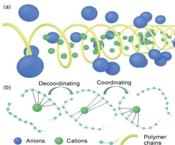
Fig. 2 Conduction mechanism of the solid polymer electrolyte. (a) Crystal vacancy diffusion model; (b) diffusion model in amorphous region.<sup>21</sup>
