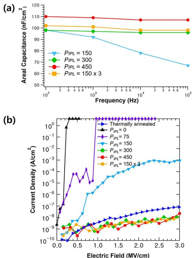
Fig. 4 Electrical characteristics of the solution-processed  $\text{AlO}_x$  thin film with varying  $P_{IPL}$ : (a) capacitance–frequency ( $C$ – $F$ ) plot. (b) Leakage current density–electric field ( $J$ – $E$ ) plot.
