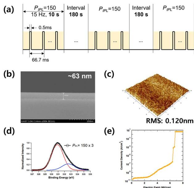
Fig. 5 (a) Schematic of  $P_{IPL} = 150 \times 3$ . Physical, chemical and electrical properties of  $\text{AlO}_x$  with  $P_{IPL} = 150 \times 3$ . (b) Cross-section SEM image. (c)  $R_{RMS}$  roughness AFM image, (d) XPS O 1s spectra, and statistical distributions of (e) the  $J$ – $E$  plot.
