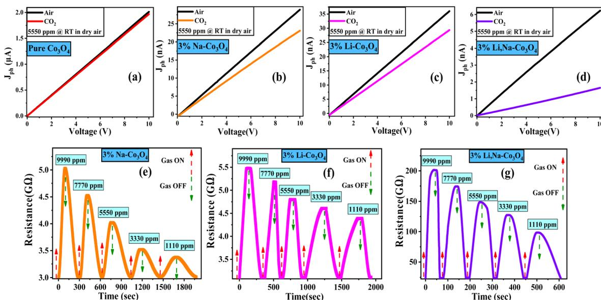
Fig. 6 Current–voltage ( $I$ – $V$ ) curves of (a) pure  $\text{Co}_3\text{O}_4$ , (b) 3% Li- $\text{Co}_3\text{O}_4$ , (c) 3% Na- $\text{Co}_3\text{O}_4$ , and (d) 3% Li, Na- $\text{Co}_3\text{O}_4$  thin films. Dynamic response of (e) 3% Li- $\text{Co}_3\text{O}_4$ , (f) 3% Na- $\text{Co}_3\text{O}_4$ , and (g) 3% Li, Na- $\text{Co}_3\text{O}_4$  thin films, and (h) the sensor response versus concentration.
