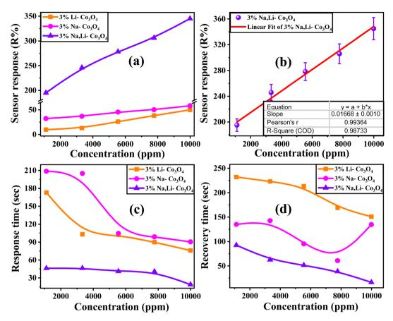
Fig. 7 (a) The sensor response of 3% Li-Co<sub>3</sub>O<sub>4</sub>, 3% Na-Co<sub>3</sub>O<sub>4</sub>, and 3% Li, Na-Co<sub>3</sub>O<sub>4</sub> thin films. (b) Linear fitted sensor response versus CO<sub>2</sub> concentration, (c) the response time, and (d) the recovery time of all Co<sub>3</sub>O<sub>4</sub> thin films vs. different gas concentrations at RT and 43% RH.
