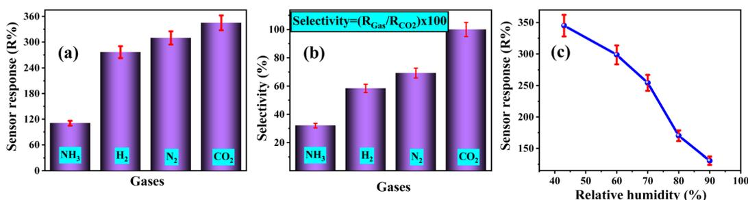
Fig. 9 (a) The sensor response and (b) selectivity of the 3% Li, Na-Co<sub>3</sub>O<sub>4</sub> sensor for several gases at 9990 ppm concentration, RT and 43% RH, and (c) sensor response under various relative humidity levels at RT.
