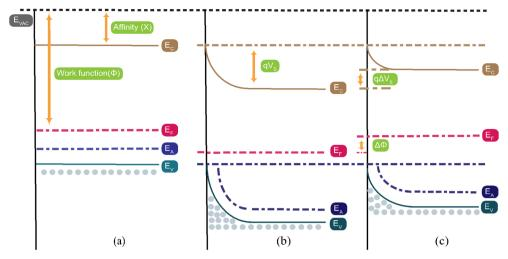
Fig. 10 The energy band structure of the  $Co_3O_4$  surface (a) before any reaction, (b) when exposed to oxygen, and (c) when  $CO_2$  gas is injected into the chamber. The term " $E_C$ " denotes the location of the conduction band, " $E_F$ " denotes the location of the Fermi level, " $E_V$ " denotes the location of the valence band, "q" denotes the charge of the electron, and " $qV_S$ " denotes the potential barrier.
