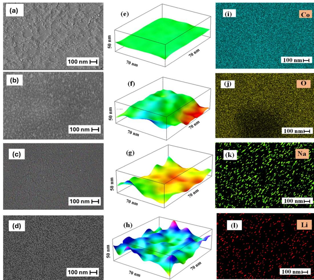
Fig. 4 SEM images for  $\text{Co}_3\text{O}_4$  thin films: (a) pure  $\text{Co}_3\text{O}_4$ , (b) 3% Li- $\text{Co}_3\text{O}_4$ , (c) 3% Na- $\text{Co}_3\text{O}_4$ , and (d) 3% Li, Na- $\text{Co}_3\text{O}_4$ . Surface roughness for  $\text{Co}_3\text{O}_4$  thin films: (e) pure  $\text{Co}_3\text{O}_4$ , (f) 3% Li- $\text{Co}_3\text{O}_4$ , (g) 3% Na- $\text{Co}_3\text{O}_4$ , and (h) 3% Li, Na- $\text{Co}_3\text{O}_4$ . (i–l) EDX elemental mapping of 3% Li, Na- $\text{Co}_3\text{O}_4$ .
