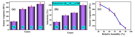
Fig. 9 (a) The sensor response and (b) selectivity of the 3% Li, Na- $Co_3O_4$  sensor for several gases at 9990 ppm concentration, RT and 43% RH, and (c) sensor response under various relative humidity levels at RT.
