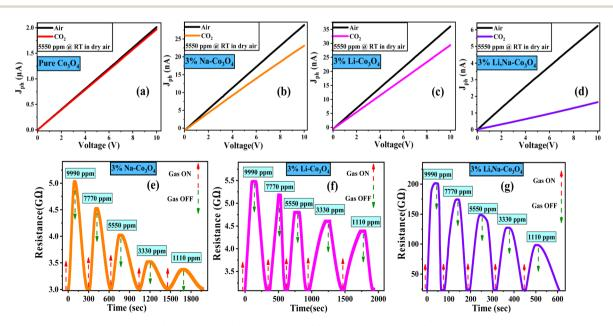
Fig. 6 Current-voltage (I-V) curves of (a) pure  $Co_3O_4$ , (b) 3% Li- $Co_3O_4$ , (c) 3% Na- $Co_3O_4$ , and (d) 3% Li, Na- $Co_3O_4$  thin films. Dynamic response of (e) 3% Li- $Co_3O_4$ , (f) 3% Na- $Co_3O_4$ , and (g) 3% Li, Na- $Co_3O_4$  thin films, and (h) the sensor response *versus* concentration.
