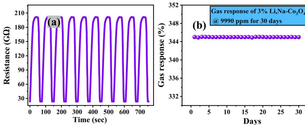
Fig. 8 (a) Repeatability and (b) stability of 3% Li, Na-Co<sub>3</sub>O<sub>4</sub> thin films at RT and 43% RH.
