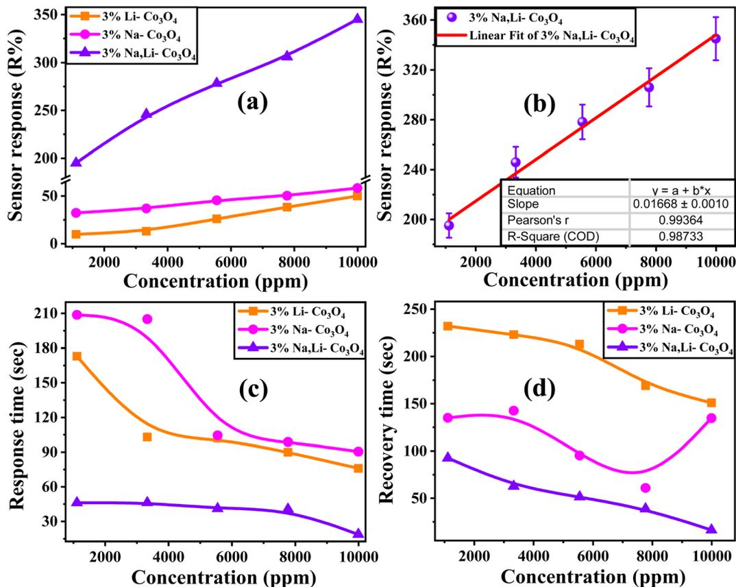
Fig. 7 (a) The sensor response of 3% Li-Co<sub>3</sub>O<sub>4</sub>, 3% Na-Co<sub>3</sub>O<sub>4</sub>, and 3% Li, Na-Co<sub>3</sub>O<sub>4</sub> thin films. (b) Linear fitted sensor response versus CO<sub>2</sub> concentration, (c) the response time, and (d) the recovery time of all Co<sub>3</sub>O<sub>4</sub> thin films vs. different gas concentrations at RT and 43% RH.
