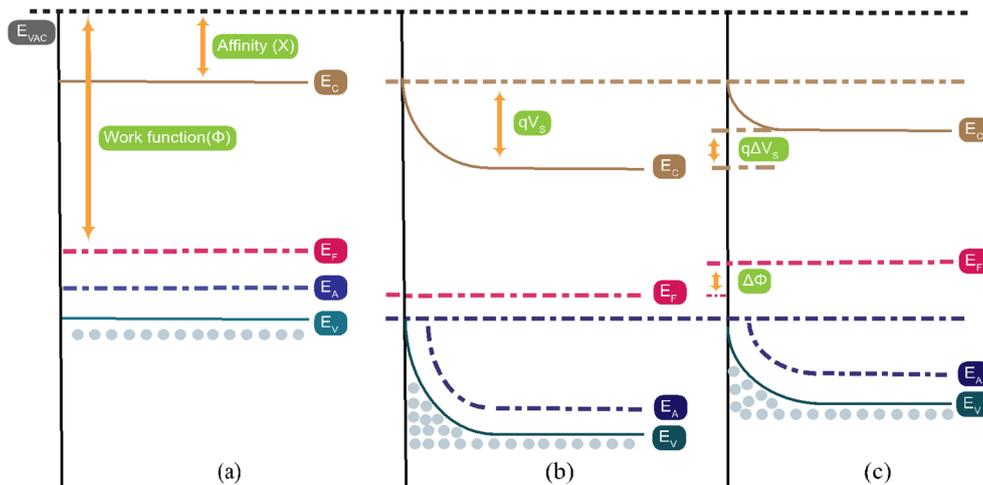
Fig. 10 The energy band structure of the  $\text{Co}_3\text{O}_4$  surface (a) before any reaction, (b) when exposed to oxygen, and (c) when  $\text{CO}_2$  gas is injected into the chamber. The term " $E_c$ " denotes the location of the conduction band, " $E_f$ " denotes the location of the Fermi level, " $E_v$ " denotes the location of the valence band, " $q$ " denotes the charge of the electron, and " $qV_s$ " denotes the potential barrier.
