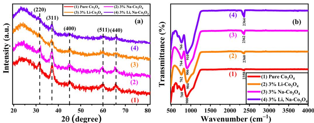
Fig. 2 (a) XRD and (b) FTIR spectra of pure Co<sub>3</sub>O<sub>4</sub>, 3% Li-Co<sub>3</sub>O<sub>4</sub>, 3% Na-Co<sub>3</sub>O<sub>4</sub>, and 3% Li, Na-Co<sub>3</sub>O<sub>4</sub> thin films.
