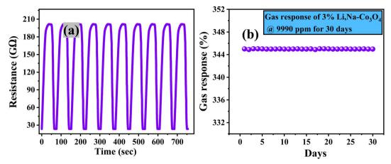
Fig. 8 (a) Repeatability and (b) stability of 3% Li, Na-Co<sub>3</sub>O<sub>4</sub> thin films at RT and 43% RH.
