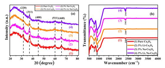
Fig. 2 (a) XRD and (b) FTIR spectra of pure  $Co_3O_4$ , 3% Li- $Co_3O_4$ , 3% Na- $Co_3O_4$ , and 3% Li, Na- $Co_3O_4$  thin films.
