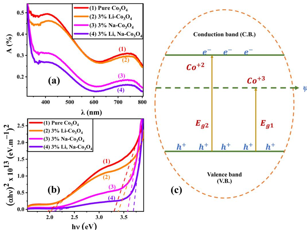
Fig. 3 (a) Absorption spectrum and (b) band gap energy plots of pure  $\text{Co}_3\text{O}_4$ , 3% Li- $\text{Co}_3\text{O}_4$ , 3% Na- $\text{Co}_3\text{O}_4$ , and 3% Li, Na- $\text{Co}_3\text{O}_4$  thin films, and (c) the band structure of  $\text{Co}_3\text{O}_4$ .
