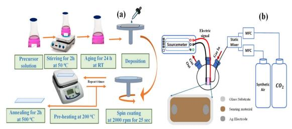
Fig. 1 The schematic of (a) spin-coating technique for the preparation of the thin films and (b) apparatus used for gas sensing measurement.
