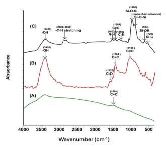
Fig. 2 FTIR spectra of (A) MWCNT, (B) -COOH CNT, and (C) GA-CNT.
