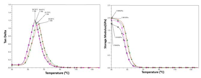
Fig. 9 Temperature variation of tan δ (left) and the storage modulus (right) in the EPB-CNT Composites with wt%: 0 (□), 1(■), 2 (●) and 4 (●).
