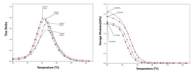
Fig. 8 Temperature variation of tan δ (left) and the storage modulus (right) in the ECB-CNT Composites with wt%: 0 (□), 1(■), 2 (♠) and 4 (♠).
