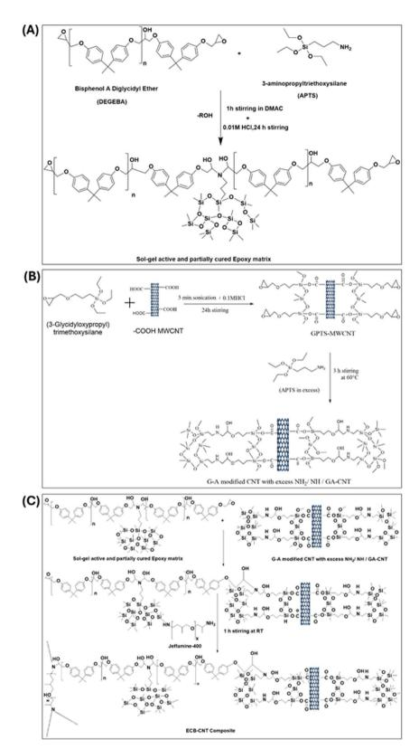
Fig. 1 (A) Preparation of (GPTS-APTS)-modified MWCNT solution/GA-CNT. (B) Preparation of the sol-gel active and partially cured polymer matrix, and (C) preparation of the ECB-CNT composite.
