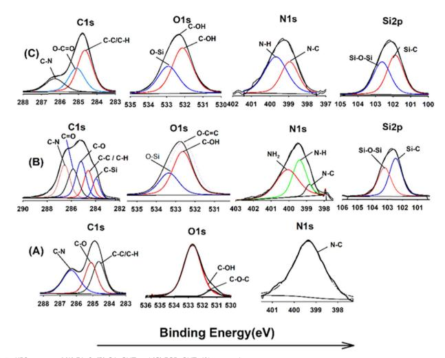
XPS spectra of (A) EA-0, (B) GA-CNT and (C) ECB-CNT-4% composites.
