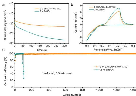
Fig. 4 (a) Comparison of chronopotentiometric tests conducted in  $\text{ZnSO}_4$  and  $\text{ZnSO}_4$  + 4 mM TAU electrolytes; (b) cyclic voltammetry curves for the electrolytes  $\text{ZnSO}_4$  and  $\text{ZnSO}_4$  + 4 mM TAU; (c) coulombic efficiency of the Zn//Cu asymmetric cells in  $\text{ZnSO}_4$  and  $\text{ZnSO}_4$  + 4 mM TAU electrolytes ( $1 \text{ mA cm}^{-2}$ ,  $0.5 \text{ mA h cm}^{-2}$ ).
