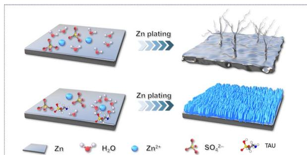
Fig. 7 Schematic diagram of the deposition behavior of Zn<sup>2+</sup> in electrolytes without and with additives.
