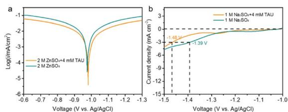
Fig. 3 (a) Tafel plots for the Zn anode in  $\text{ZnSO}_4$  and  $\text{ZnSO}_4$  + 4 mM TAU electrolytes; (b) linear sweep voltammetry curves for the anode in  $\text{Na}_2\text{SO}_4$  and  $\text{Na}_2\text{SO}_4$  + 4 mM TAU electrolytes.
