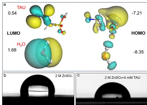
Fig. 1 (a) Energy levels of the highest occupied molecular orbital (HOMO) and the lowest unoccupied molecular orbital (LUMO) for TAU and  $\text{H}_2\text{O}$ ; (b) contact angle of  $\text{ZnSO}_4$  electrolyte on the surface of the Zn anode; (c) contact angle of  $\text{ZnSO}_4$  electrolyte containing 4 mM TAU on the surface of the Zn anode.
