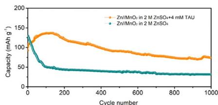
Fig. 6 Comparison of cycling performance for the Zn//MnO<sub>2</sub> full cell in different electrolytes.
