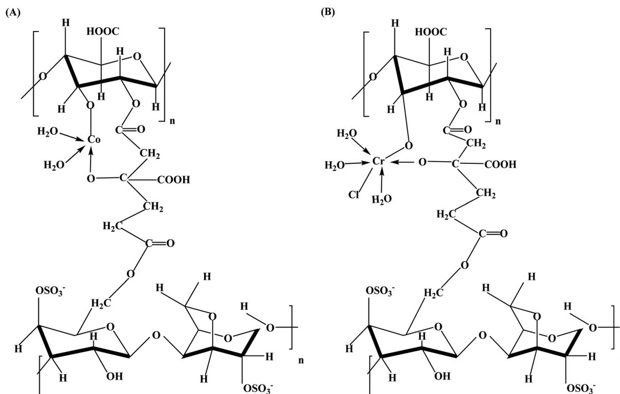
**Fig. 2** Proposed structures of the complex (A) [Co(AG/CTR/CAR)(H<sub>2</sub>O)<sub>2</sub>], and the complex (B) [Cr(AG/CTR/CAR)(H<sub>2</sub>O)<sub>3</sub>Cl].
