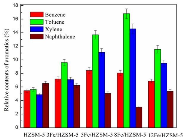
Fig. 7 Content of aromatics with different Fe loadings.
