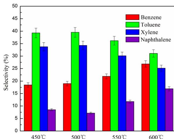
Fig. 11 Selectivity of aromatics at different temperatures.
