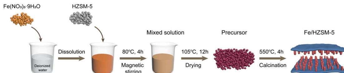
Fig. 1 Preparation processes of Fe-modified HZSM-5 catalysts.
