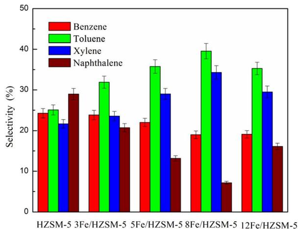
Fig. 8 Selectivity of aromatics with different Fe loadings.
