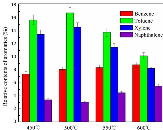
Fig. 10 Content of aromatics at different temperatures.
