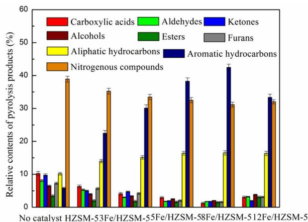
Fig. 6 Pyrolysis product content with different Fe loading.
