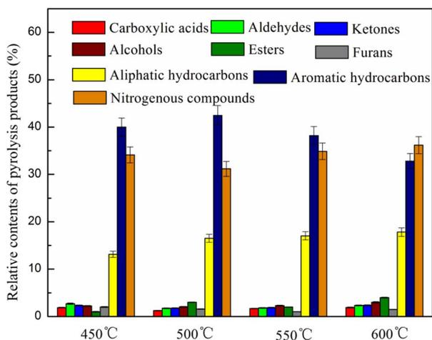
Fig. 9 Pyrolysis product content at different temperatures.
