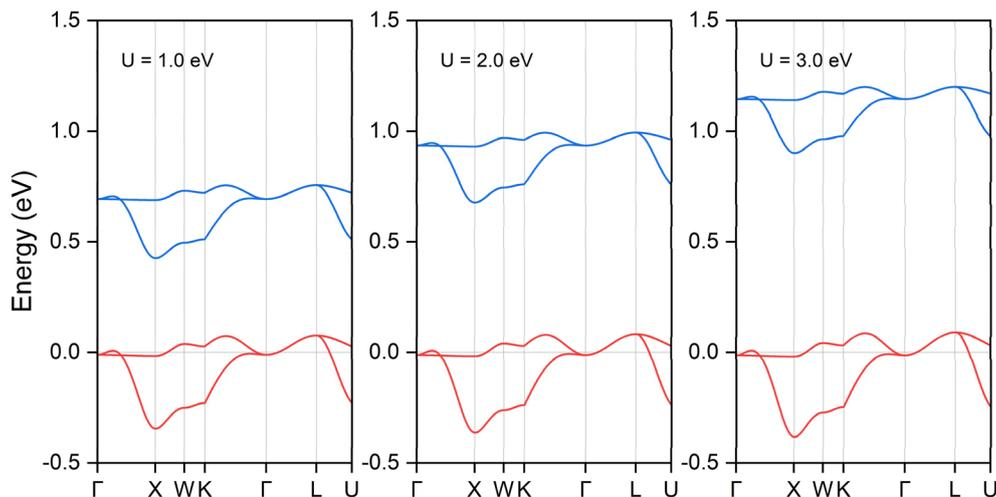
Fig. 4 The local band structure in both spin channels along the  $\Gamma$ -X-W-K- $\Gamma$ -L-U path for ternary ferromagnetic compound  $K_3NiCl_6$  under DFT +  $U$  method. The Fermi energy level is shifted to 0 eV, as indicated by the horizontal line. Hubbard  $U$  values ranging from 1 to 3 eV were employed to accommodate strong Coulomb interactions. Only the bands related to the spin nodal box are shown.
