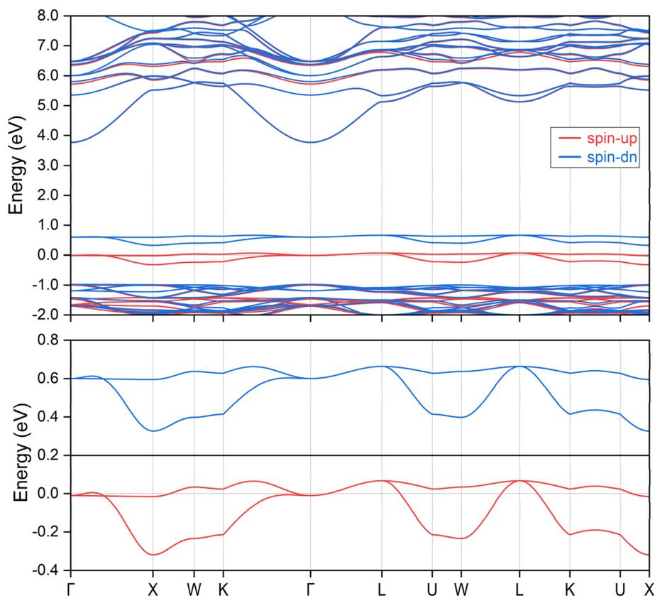
Fig. 2 The spin polarized electronic band structures for the ternary ferromagnetic compound  $\text{K}_3\text{NiCl}_6$ . The Fermi energy level is shifted to 0 eV, as indicated by the horizontal line. Two local band structures in proximity to the Fermi energy level are further magnified at the bottom panel, in which multiple band crossings can be clearly observed.
