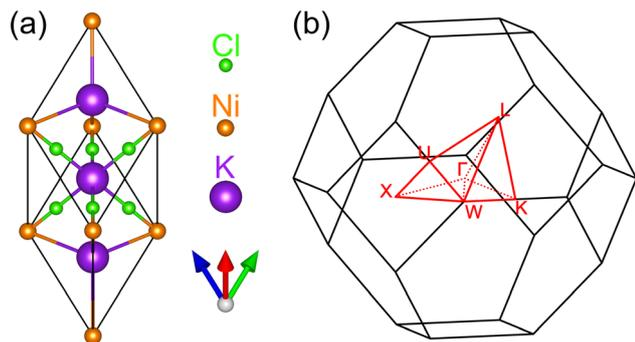
Fig. 1 The primitive cell (a) and the corresponding Brillouin zone (b) for the ternary ferromagnetic compound  $\text{K}_3\text{NiCl}_6$ . The high symmetry paths and points are highlighted in red for clarity.
