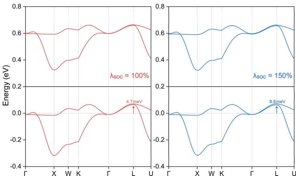
Fig. 5 The calculated local band structure along the  $\Gamma$ -X-W-K- $\Gamma$ -L-U path for ternary ferromagnetic compound  $K_3NiCl_6$  under the influence of spin-orbit coupling effect. The Fermi energy level is shifted to 0 eV, as indicated by the horizontal line. Furthermore, the coupling intensity has been artificially increased to investigate extreme scenarios. The maximum opened band gap is situated at the L point, with the corresponding gap value explicitly indicated.
