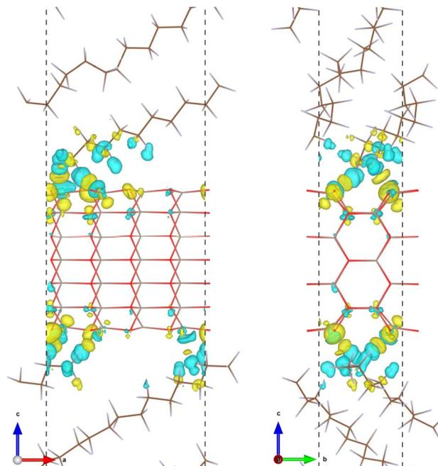
Fig. 3 Isosurface view of electron density difference at the value of  $0.001|e| \text{ \AA}^{-3}$  upon the interface formation of ZnO/a-PTFE model1 with a ZnO fraction of 33.67 wt%. The yellow (cyan) color represents the charge accumulation (depletion).
