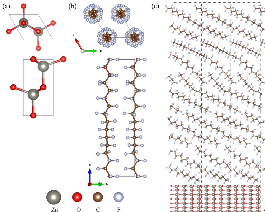
Fig. 1 Ball-and-stick views of (a) a bulk ZnO unit cell in the hexagonal phase (space group  $P6_3mc$ ), (b) a c-PTFE unit cell in the hexagonal phase (space group  $P31$ ), and (c) ZnO/a-PTFE supercells composed of a ZnO (1120) surface ( $2 \times 1$ ) supercell with 7 atomic layers and a-PTFE polymers filled in a 65 Å height space (33.67 wt% ZnO), where the dashed lines indicate the lattice.
