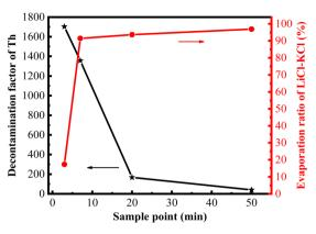
Fig. 6 Evaporation ratio of LiCl–KCl and decontamination factor of Th at different evaporation times.
