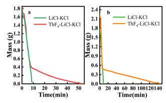
Fig. 2 Mass loss curves under vacuum distillation conditions at 1173 K and 20 Pa: (a) 1.8 g of 20 wt% ThF $_4$ -LiCl-KCl and 1.8 g of LiCl-KCl; (b) 2.25 g of 20 wt% ThF $_4$ -LiCl-KCl and 1.8 g of LiCl-KCl.
