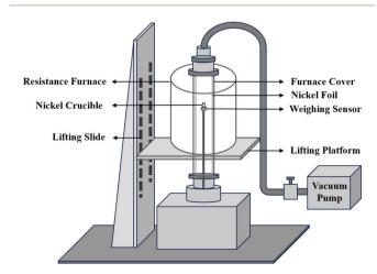
Fig. 1 A Schematic diagram of vacuum distillation apparatus.
