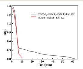
Fig. 7 Weight loss curves of 20 wt% ThF $_4$ -1 wt% SmF $_3$ -1 wt% NdF $_3$ -LiCl-KCl mixed salt.
