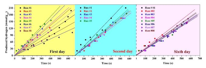
Fig. 11 Stability of the proposed treated nanofibers as a photocatalyst for hydrogen generation from methanol/water solution (70% methanol) under solar radiation within 6 days working time.
