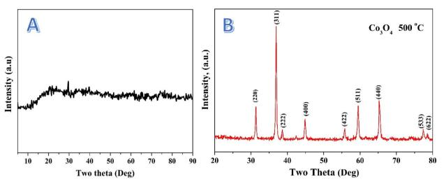
Fig. 3 XRD patterns for the treated; (A) and Co<sub>3</sub>O<sub>4</sub>; (B) nanofibers
