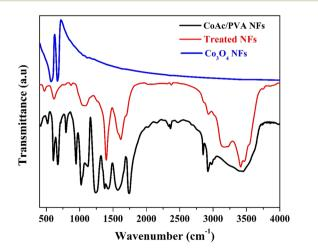
Fig. 4 FTIR spectra of the original CoAc/PVA electrospun nanofibers, the treated nanofibers and  $Co_3O_4$  nanofibers.
