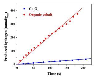
Fig. 9 Hydrogen generation rate from methanol/water solution (50% methanol) under visible radiation using the treated and Co<sub>3</sub>O<sub>4</sub> nanofibers.
