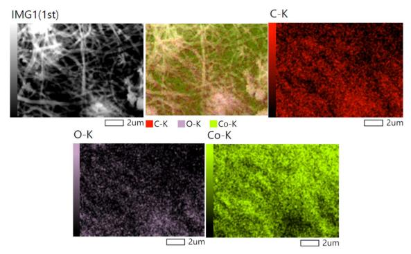
Elemental mapping analyses for the treated nanofibers
