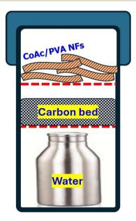
Fig. 1 Schematic diagram for the used reactor for preparation the organic cobalt nanofibers.
