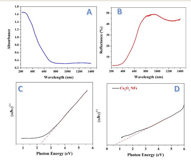
Fig. 8 Absorbance *versus* wavelength; (A) and reflectance *versus* wavelength; (B) for the treated nanofibers. Tauc plot of photons energy at direct band gap energy as function of  $(\alpha h \nu)^2$  for the treated nanofibers; (C) and  $Co_3O_4$  nanofibers; (D).
