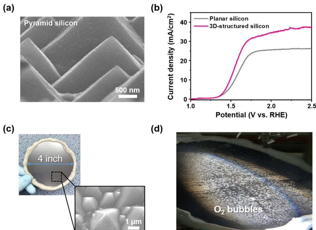
**Fig. 3** (a) An SEM image of CBD NiO coating on the 3D-structured silicon substrate. (b) Plots of photocurrent density vs. voltage using NiO films deposited on 3D-structured (red) and planar (grey) n-Si substrates. (c) Optical photograph of CBD NiO coating on the 3D-structured 4-inch silicon substrate and (d) photoelectrochemical water splitting (oxygen bubbling) therein under light illumination (see also the ESI Movie†).
