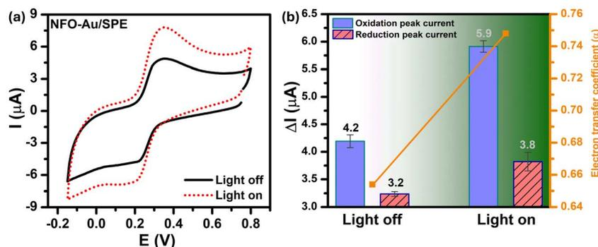
Fig. 3 (a) CV curves and (b) the corresponding bar diagram of oxidation/reduction peak currents and the electron transfer coefficient of Au-NFO/SPE in 0.1 M PBS (pH 7.0) solution containing  $50 \mu M$  PCM in the absence and presence of visible light. The scan rate of CV is  $50 mV s^{-1}$ .
