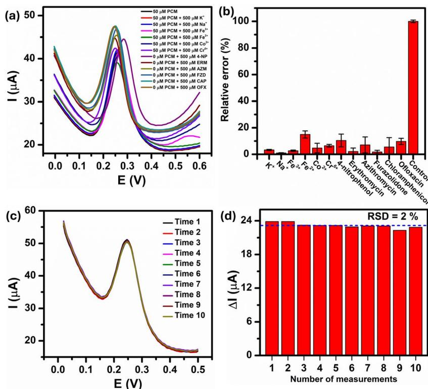
**Fig. 9** (a and b) Interference investigation of Au–NFO/SPE in 0.1 M PBS solution containing 100  $\mu\text{M}$  PCM with 10-fold concentration of interference substances and (c and d) the repeatability performance of Au–NFO/SPE for 10 consecutive measurements in 0.1 M PBS solution containing 100  $\mu\text{M}$  PCM.
