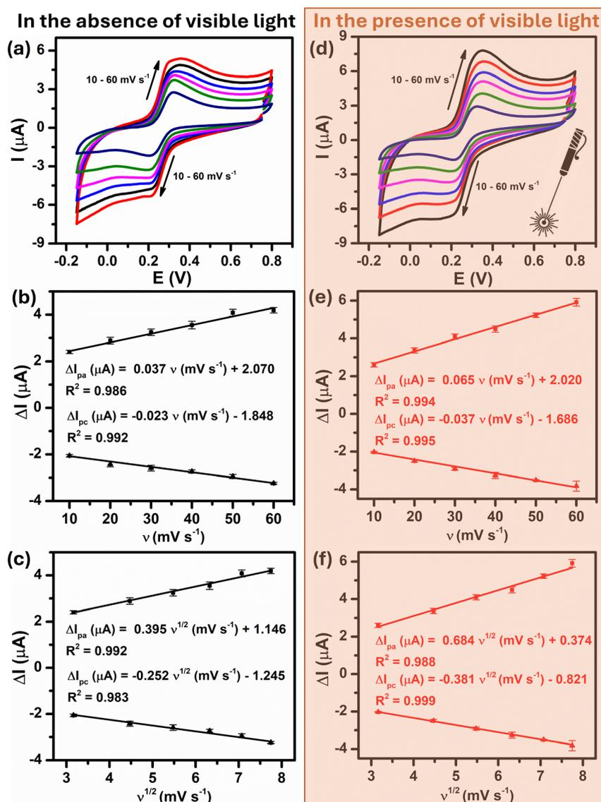
Fig. 4 CV curves of Au-NFO/SPE recorded at various scan rates from 10 to 60  $\text{mV s}^{-1}$ , the corresponding calibration plots of oxidation/reduction peak current vs. scan rate and the square root of scan rate in the absence (a–c) and in the presence (d–f) of visible light, respectively.
