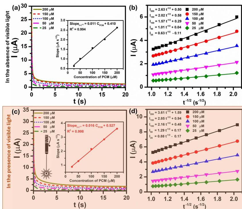
Fig. 5 CA curves of Au-NFO/SPE in  $0.1 \text{ M}$  PBS (pH 7.0) solution containing different concentrations of PCM (25, 50, 100, 150, and  $200 \mu\text{M}$ ) and plot of  $I$  *vs.*  $t^{-1/2}$  in the absence (a and b) and presence (c and d) of visible light, respectively. Inset the plot of the slope of the straight lines against PCM concentration.
