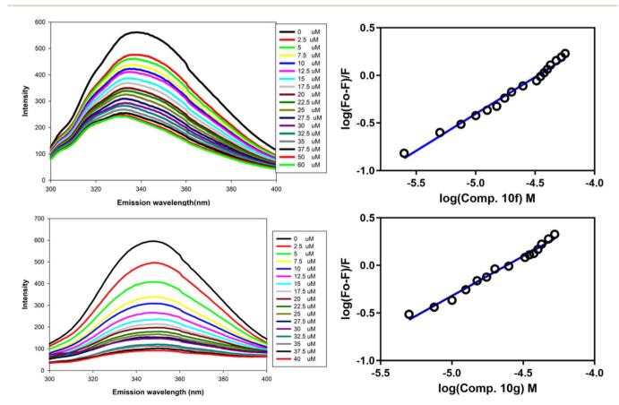
Fig. 4 Fluorescence spectra of compound 10f (top panel) and 10g (bottom panel).
