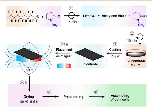
Scheme 1 Cathode preparation procedure.
