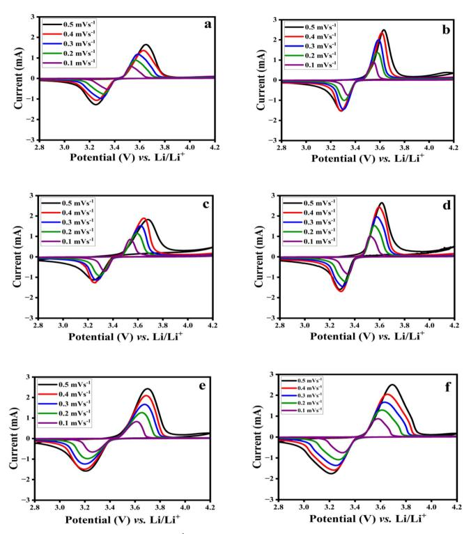
Fig. 4 CV curves at various rates from 0.1 to 0.5 mV s<sup>-1</sup> for (a) LFP, (b) LFP-MF, (c) 1% FO/LFP, (d) 1% FO/LFP-MF, (e) 3% FO/LFP, and (f) 3% FO/LFP-MF.
