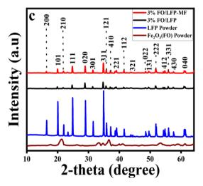
Fig. 1 XRD patterns of the cathodes: (a) LFP and LFP-MF; (b) 1% FO/LFP and 1% FO/LFP-MF; and (c) 3% FO/LFP and 3% FO/LFP-MF.
