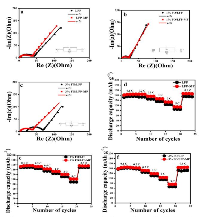
Fig. 5 (a) Nyquist plots of AC impedance spectra for LFP and LFP-MF; (b) 1% FO/LFP and 1% FO/LFP-MF; and (c) 3% FO/LFP and 3% FO/LFP-MF. Comparison of the rate capacity data for (d) LFP and LFP-MF; (e) 1% FO/LFP and 1% FO/LFP-MF; and (f) 3% FO/LFP and 3% FO/LFP-MF.
