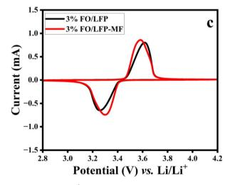
Fig. 3 (a) CV scans ( $4^{th}$  cycle) of LFP and LFP-MF; (b) 1% FO/LFP and 1% FO/LFP-MF; and (c) 3% FO/LFP and 3% FO/LFP-MF.
