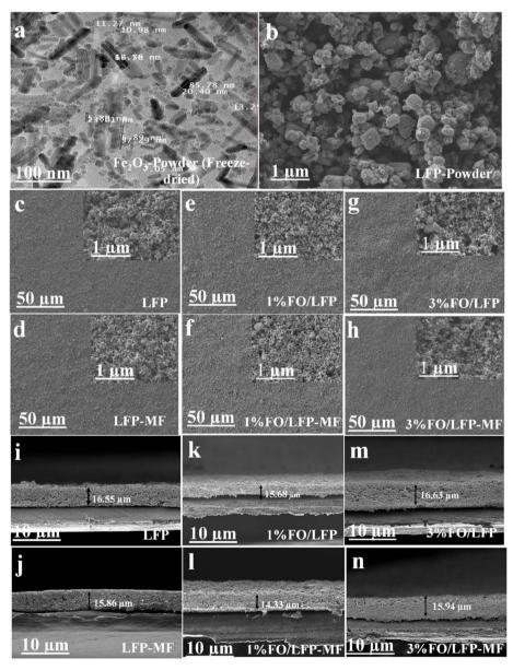
Fig. 2 (a) TEM image of freeze-dried  $Fe_2O_3$  nanoparticles; (b) top-view SEM images of LiFePO<sub>4</sub> powder; (c) LFP and (d) LFP-MF; (e) 1% FO/LFP and (f) 1% FO/LFP-MF; and (g) 3% FO/LFP and (h) 3% FO/LFP-MF cathodes; cross-sectional SEM images of cathodes (i) LFP and (j) LFP-MF; (k) 1% FO/LFP and (l) 1% FO/LFP-MF; (m) 3% FO/LFP and (n) 3% FO/LFP-MF.
