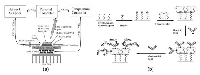
Fig. 6 Schematic structure of (a) dip-and-dry test<sup>101</sup> and (b) immunochemical reactions and biomolecule additions on the LGS SH-SAW sensor with phase changes.<sup>102</sup>
