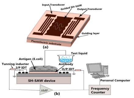
Fig. 4 Schematic representation of the SH-SAW delay-line.91
