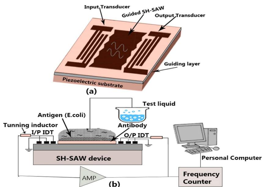
Fig. 4 Schematic representation of the SH-SAW delay-line.<sup>91</sup>
