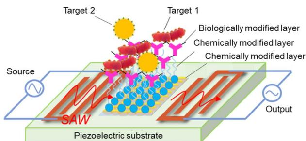
Fig. 1 Basic structure of a SAW biosensor.
