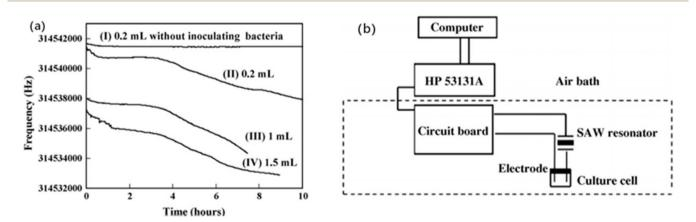
Fig. 8 (a) Effect of sample volume on the response of the SAW sensor. The sample was a nutrient broth (pH 7.0) inoculated with about 105 cells per mL *E. coli.* (b) New surface acoustic wave sensor for microbial count monitoring in biological cultures at ultrahigh frequencies.<sup>114</sup>
