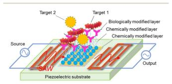
Fig. 1 Basic structure of a SAW biosensor.
