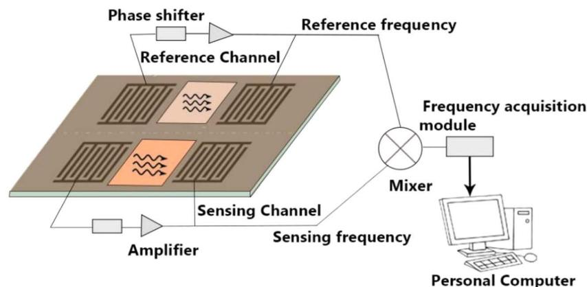
Fig. 9 Schematic of a dual-channel SAW sensor.
