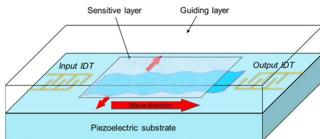
Fig. 2 Basic structure of a Love-wave surface acoustic wave sensor.
