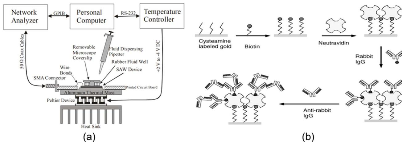
Fig. 6 Schematic structure of (a) dip-and-dry test<sup>101</sup> and (b) immunochemical reactions and biomolecule additions on the LGS SH-SAW sensor with phase changes.<sup>102</sup>
