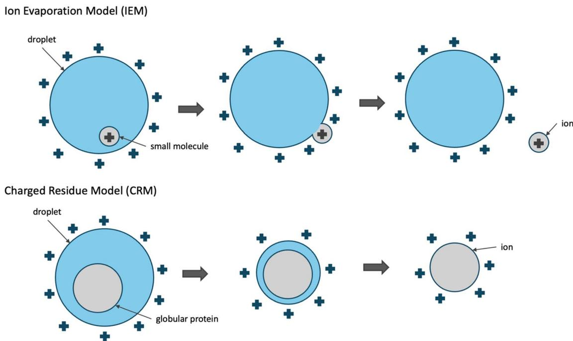
Fig. 1 Conceptual models describing the mechanism of electrospray ionization. Small molecules are thought to be ionized through the ion evaporation model (IEM),<sup>15</sup> while larger molecules, such as globular proteins are thought to ionize through the charged residue model (CRM).<sup>15</sup>
