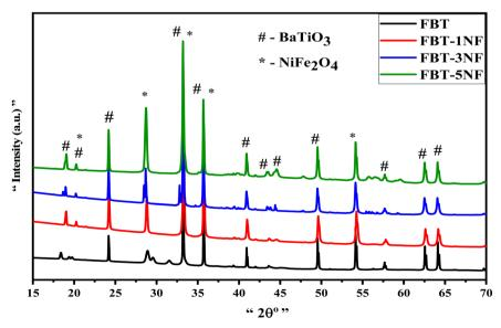
Fig. 1 XRD patterns of nano hexagonal Fe<sub>0.3</sub>BaTi<sub>0.7</sub>O<sub>3</sub> coated by (1, 3, 5) NF composites.
