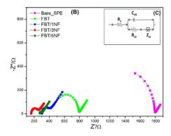
Fig. 7 (A) CV measurements of unmodified (bare) SPE, FBT, FBT/1NF, FBT/3NF and FBT/5NF modified SPEs were conducted in a solution of standard redox probe of 5 mM ferricyanide and 0.1 M KCl as the supporting electrolyte. Scan rate of 50 mV s<sup>-1</sup> was applied for all experiments. (B) EIS Nyquist spectra characterization of unmodified and modified electrodes with the nanomaterials. (C) The inset represents the modeled circuit that is used for curve fitting.
