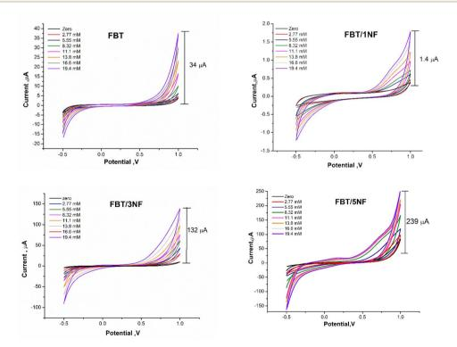
Fig. 10 CVs response of GOx@GA@FBT/NF@SPEs biosensor's containing different ratios of FBT/xNF nanocomposites (FBT; FBT:1NF; FBT:3NF; or FBT:5NF) and fixed concentration of GOx with500  $\mu$ g ml<sup>-1</sup> and 2.5% GA. The voltametric scans was carried out by using PBS buffer (pH = 7.4) solution containing different concentrations of glucose from 2.77–19.4 mM.
