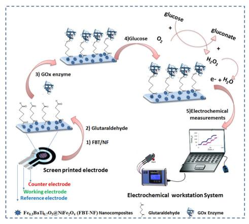
Scheme 1 A simple demonstration presented the steps of glucose biosensor preparations showing the chemical immobilization of the active enzyme (GOx) though the crosslinking with the glutaraldehyde molecules. Oxidation of glucose to gluconic acid and generation of peroxide as an electrochemically active bi-product to be oxidized at the active nanomaterial substrate.
