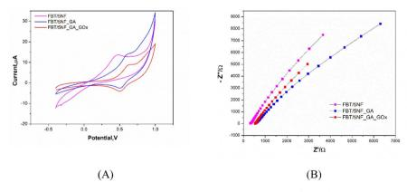
Fig. 9 (A) CV and (B) EIS measurements of the GOx enzyme immobilization steps on the FBT/5NF@SPE surface in a solution containing standard redox probe of 5 mM ferricyanide and KCl as the supporting electrolyte. Scan rate of 50 mV s<sup>-1</sup> was applied for all experiments.
