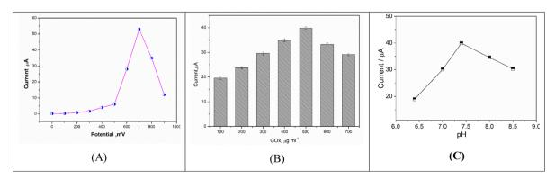
Fig. 12 (A) Effect of accumulation potential on the chronoamperometric current responses of the GOx-based biosensor in a solution of PBS (pH = 7.4) containing 0.83 mM glucose. (B) Effect of GOx concentration on the biosensor current response by using PBS buffer (pH = 7.4) containing 0.69 mM of glucose. (C) Effect of different pHs of phosphate buffer on the glucose biosensors current response in the presence of glucose with a concentration of 0.69 mM.
