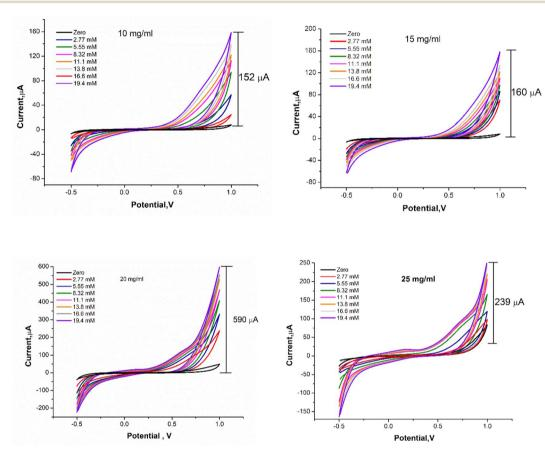
Fig. 11 CVs response of GOx@GA@FBT/5NF@SPEs biosensor's containing different concentrations (10,15,20 and 25 mg ml $^{-1}$ ) of FBT/5NF nanocomposite and fixed concentration of GOx with500  $\mu$ g ml $^{-1}$  and 2.5% GA. The voltammetric scans was carried out by using PBS buffer (pH = 7.4) solution containing different concentrations of glucose from 2.77-19.4 mM.
