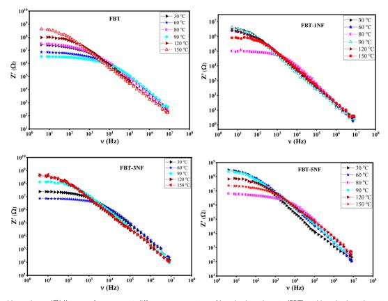
Fig. 4 The real impedance (Z'(v)) versus frequency at different temperature of iron barium titanate (FBT) and iron barium titanate shielded with nickel ferrite (FBT/xNF).
