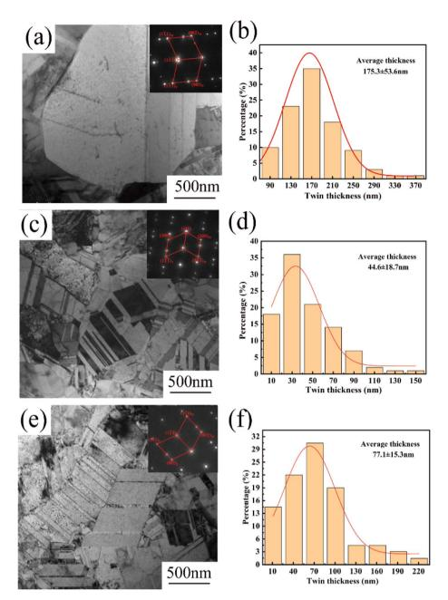
Fig. 5 TEM images and the corresponding twin thickness distributions of copper foils prepared with various PEG concentrations: (a and b)  $0 \text{ mg L}^{-1}$ , (c and d)  $4 \text{ mg L}^{-1}$  and (e and f)  $6 \text{ mg L}^{-1}$ .
