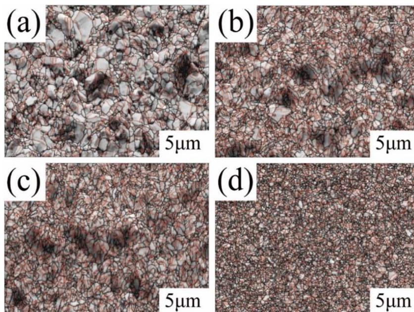
Fig. 4 Distribution of  $\Sigma 3$  grain boundaries in copper foils with various PEG concentrations: (a) 0 mg L<sup>-1</sup>, (b) 2 mg L<sup>-1</sup>, (c) 4 mg L<sup>-1</sup>, and (d) 6 mg L<sup>-1</sup>.
