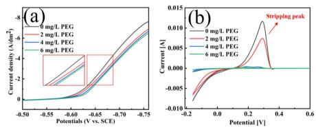
Fig. 7 LSV (a) and CV (b) curves from different concentrations of PEG in the plating solution.
