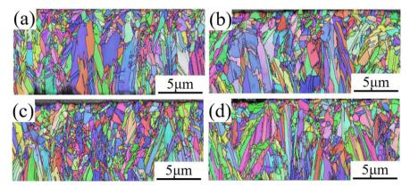
Fig. 8 Cross-sectional EBSD images of copper foils prepared with different PEG concentrations: (a) 0 mg L; (b) 2 mg L; (c) 4 mg L; (d) 6 mg L<sup>-1</sup>.
