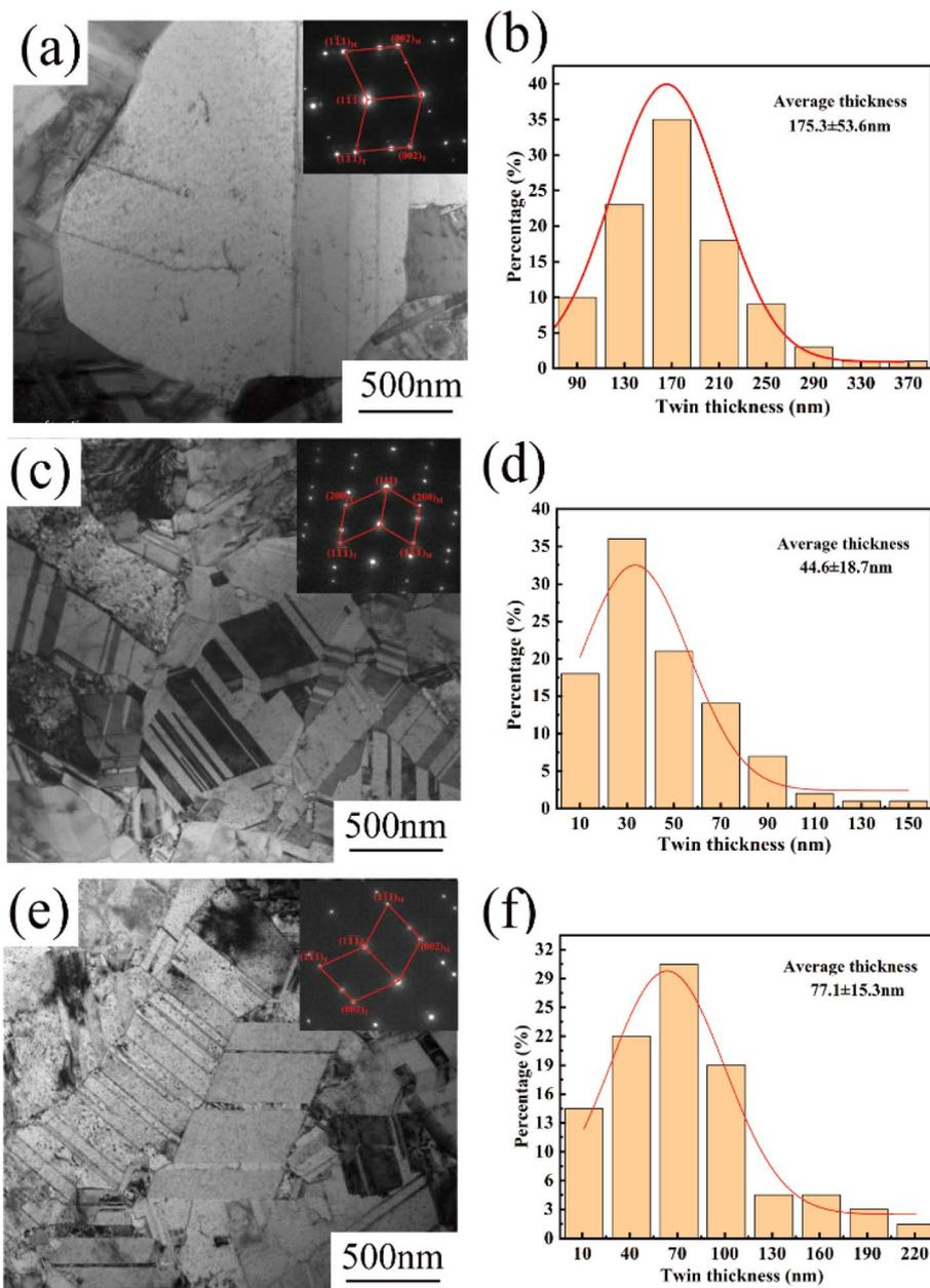
Fig. 5 TEM images and the corresponding twin thickness distributions of copper foils prepared with various PEG concentrations: (a and b)  $0 \text{ mg L}^{-1}$ , (c and d)  $4 \text{ mg L}^{-1}$  and (e and f)  $6 \text{ mg L}^{-1}$ .
