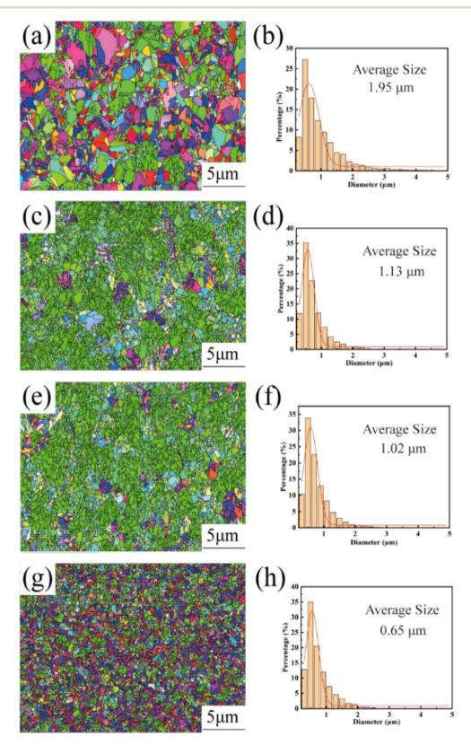
Fig. 3 EBSD plots and corresponding grain size distributions on the surface of copper foils prepared with different PEG concentrations: (a and b) 0 mg  $L^{-1}$ ; (c and d) 2 mg  $L^{-1}$ ; (e and f) 4 mg  $L^{-1}$ ; (g and h) 6 mg  $L^{-1}$ .
