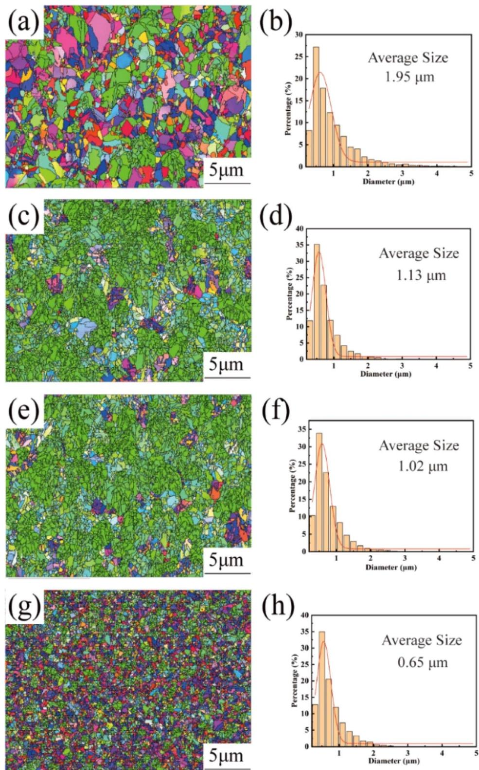
Fig. 3 EBSD plots and corresponding grain size distributions on the surface of copper foils prepared with different PEG concentrations: (a and b)  $0 \text{ mg L}^{-1}$ ; (c and d)  $2 \text{ mg L}^{-1}$ ; (e and f)  $4 \text{ mg L}^{-1}$ ; (g and h)  $6 \text{ mg L}^{-1}$ .
