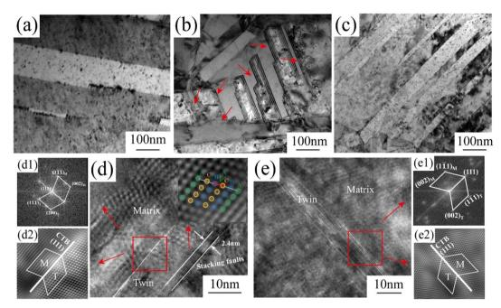
Fig. 6 High-magnification TEM (a – c) and HRTEM (d and e) images of copper foils prepared by adding 0 mg  $L^{-1}$  (a), 4 mg  $L^{-1}$  (b, d, d1, and d2) and 6 mg  $L^{-1}$  (c, e, e1, and e2) PEG, and the corresponding plots obtained in the FFT mode (d1 and e1) and IFFT mode (d2 and e2).
