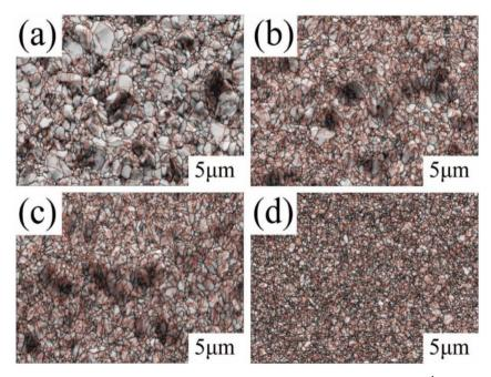
Fig. 4 Distribution of  $\sum 3$  grain boundaries in copper foils with various PEG concentrations: (a) 0 mg L<sup>-1</sup>, (b) 2 mg L<sup>-1</sup>, (c) 4 mg L<sup>-1</sup>, and (d) 6 mg L<sup>-1</sup>.
