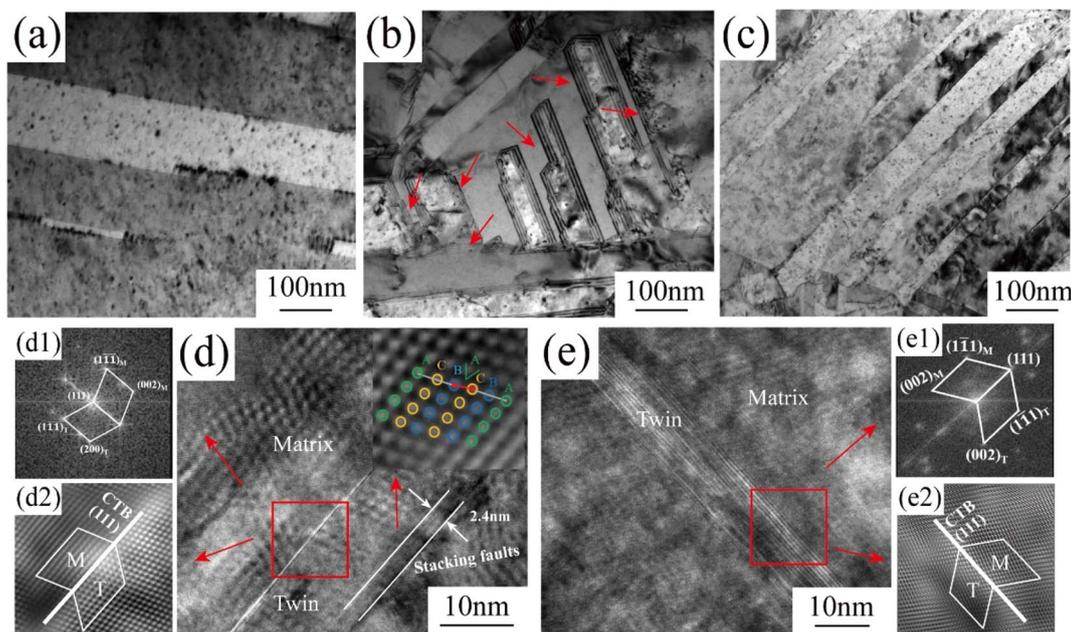
Fig. 6 High-magnification TEM (a–c) and HRTEM (d and e) images of copper foils prepared by adding 0 mg L<sup>-1</sup> (a), 4 mg L<sup>-1</sup> (b, d, d1, and d2) and 6 mg L<sup>-1</sup> (c, e, e1, and e2) PEG, and the corresponding plots obtained in the FFT mode (d1 and e1) and IFFT mode (d2 and e2).
