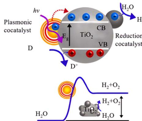
Fig. 1 Principle of photocatalytic oxidation of TiO<sub>2</sub> nanoparticles.<sup>14</sup>
