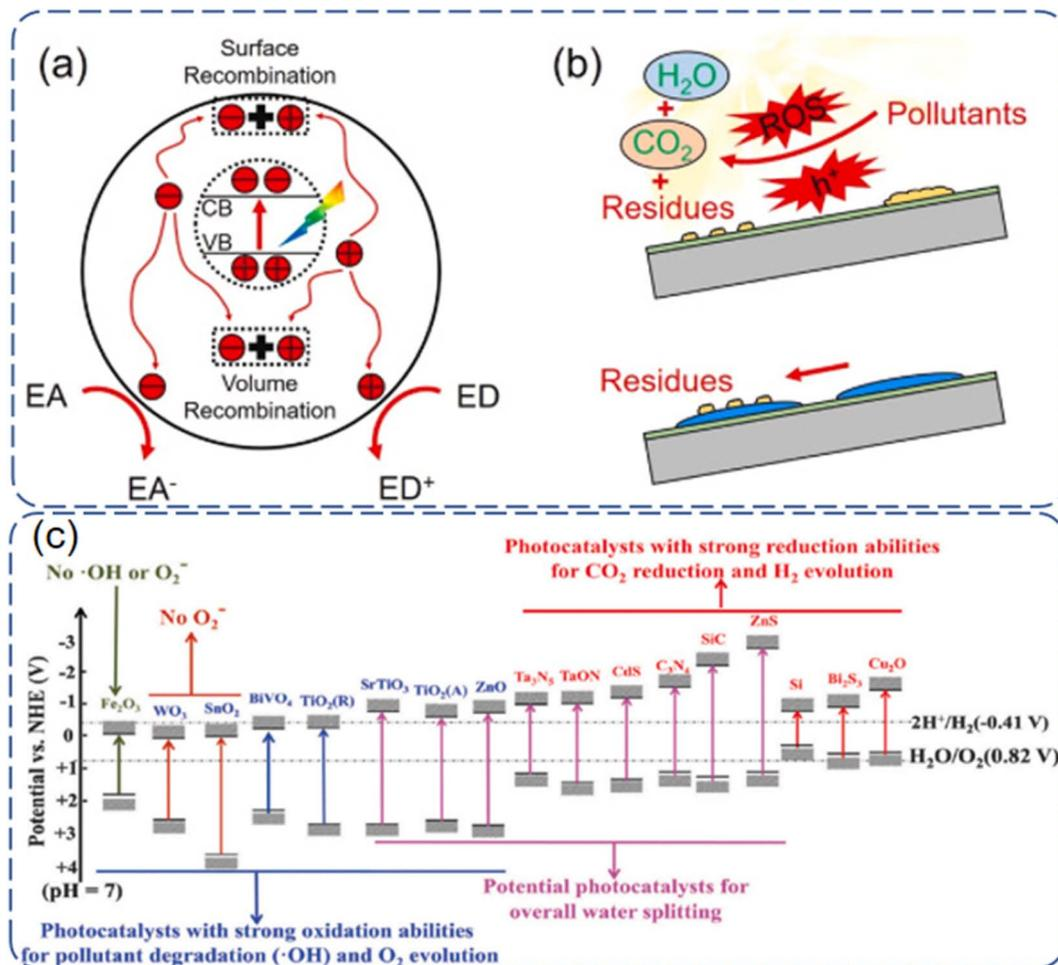
Fig. 2 Schematic illustration of (a) photoexcited charges in with possible action pathways and (b) photocatalytic self-cleaning principle.<sup>15</sup> (c) Conduction band and valence band values of some typical photocatalysts.<sup>16</sup>
