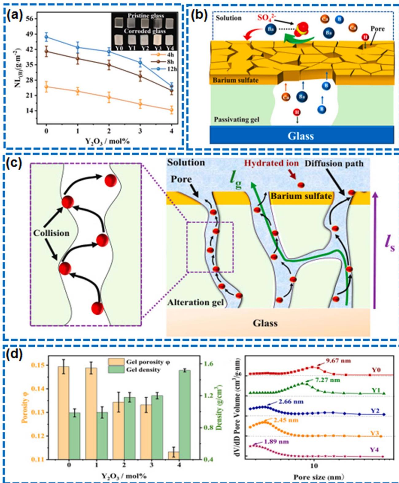
Fig. 14 (a) The effect of  $Y_2O_3$  doping on acid resistance of the glass. (b) Schematic diagram of ion diffusion in passivating gel. (c) Schematic diagram of hydrated ion diffusion in passivating gel. (d) Density and porosity of alteration products and Pore size distribution of the alteration products.<sup>158</sup>
