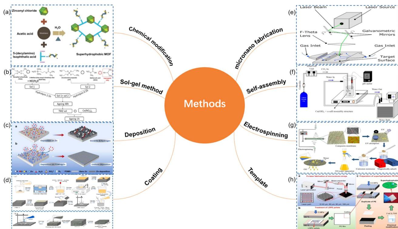
Fig. 4 Preparation method of superhydrophobic surface: (a) chemical modification;<sup>33,34</sup> (b) sol–gel method;<sup>35,36</sup> (c) deposition;<sup>37,38</sup> (d) coating;<sup>39–42</sup> (e) micronano fabrication;<sup>43,44</sup> (f) self-assembly;<sup>45,46</sup> (g) electrospinning;<sup>47,48</sup> (h) template<sup>49,50</sup>
