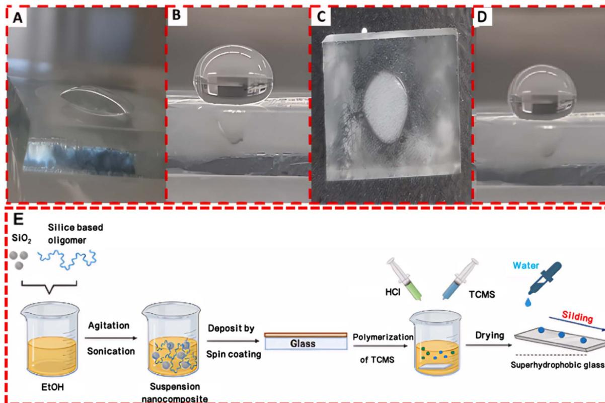
Fig. 13 Anti-icing test: (A) bare surface at  $t_0$ , (B) coated surface at  $t_0$ , (C) bare surface after 20 min at  $-10\text{ }^\circ\text{C}$ , (D) coated surface after 20 min at  $-10\text{ }^\circ\text{C}$ . (E) Schematic illustration of the preparation of the transparent superhydrophobic coating.<sup>153</sup>
