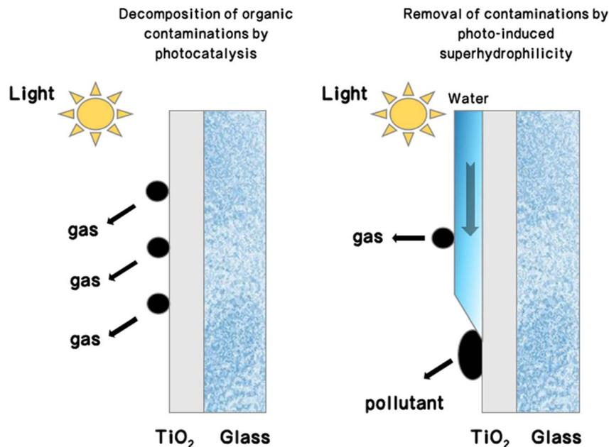
Fig. 7 Schematic illustration of the self-cleaning process on  $\text{TiO}_2$  glass surfaces with photocatalytic activity and photo-induced superhydrophilicity.<sup>14,69</sup>
