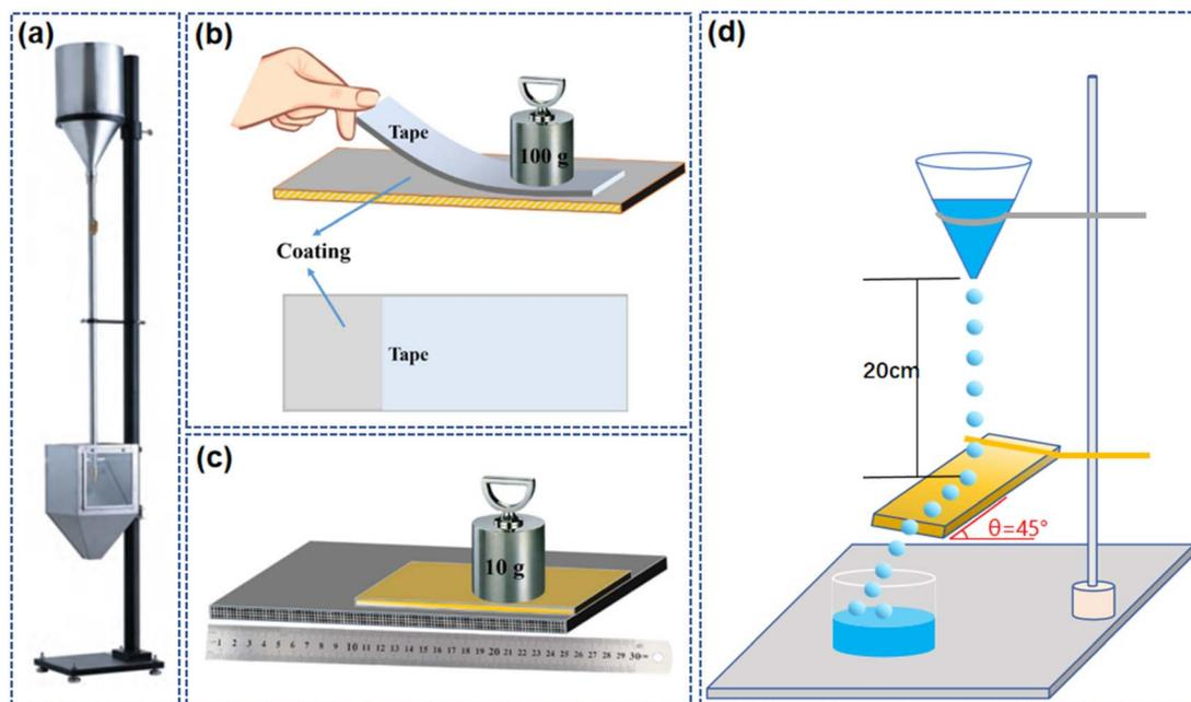
Fig. 10 Test method for robustness of self-cleaning coating: (a) sand falling test.<sup>114,115</sup> Tape peeling test (b) and sandpaper abrasion test (c).<sup>111</sup> (d) Water-impacting test.<sup>116</sup>
