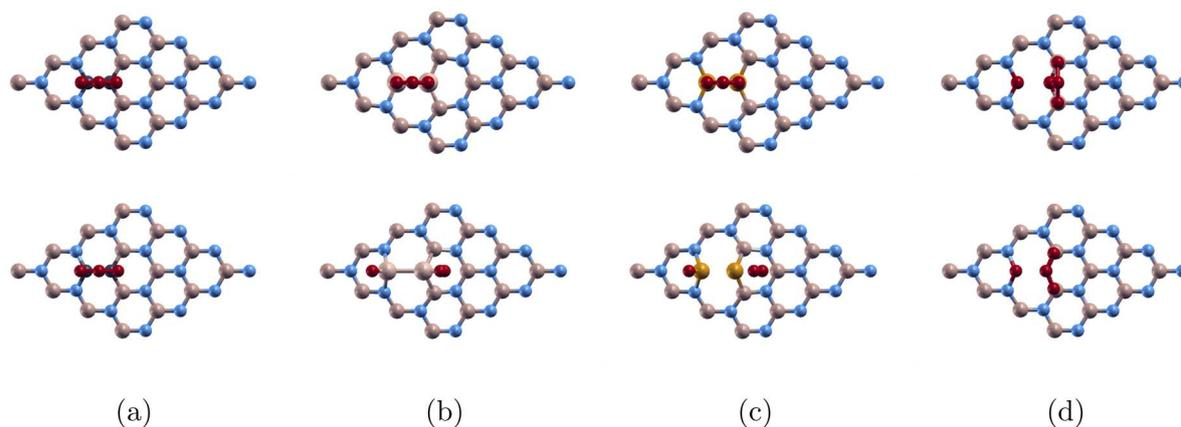
Fig. 4 Ozone adsorbed on doped monolayers before and after optimization: top row and bottom row shows atomic structure before and after optimization respectively for (a)  $O_3/C$ -BN, (b)  $O_3/Si$ -BN, (c)  $O_3/P$ -BN, and (d)  $O_3/O$ -BN. Color code as following: boron atoms, nitrogen atoms, carbon atoms, silicon atoms, phosphorus atoms, and oxygen atoms are colored beige, blue, black, white, yellow and red respectively.
