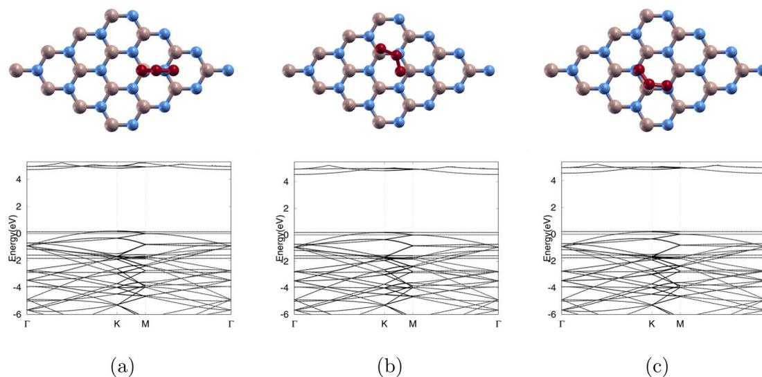
Fig. 3 Ozone adsorbed on pure monolayers in 3 different positions: top row shows atomic structures and bottom row shows band structures for (a)  $\text{BN-T}_{\text{BN}}$ , (b)  $\text{BN-T}_{\text{BB}}$ , and (c)  $\text{BN-T}_{\text{NN}}$ . 0 eV is the Fermi level. Color code as following: boron atoms, nitrogen atoms, and oxygen atoms are beige, blue, and red respectively.
