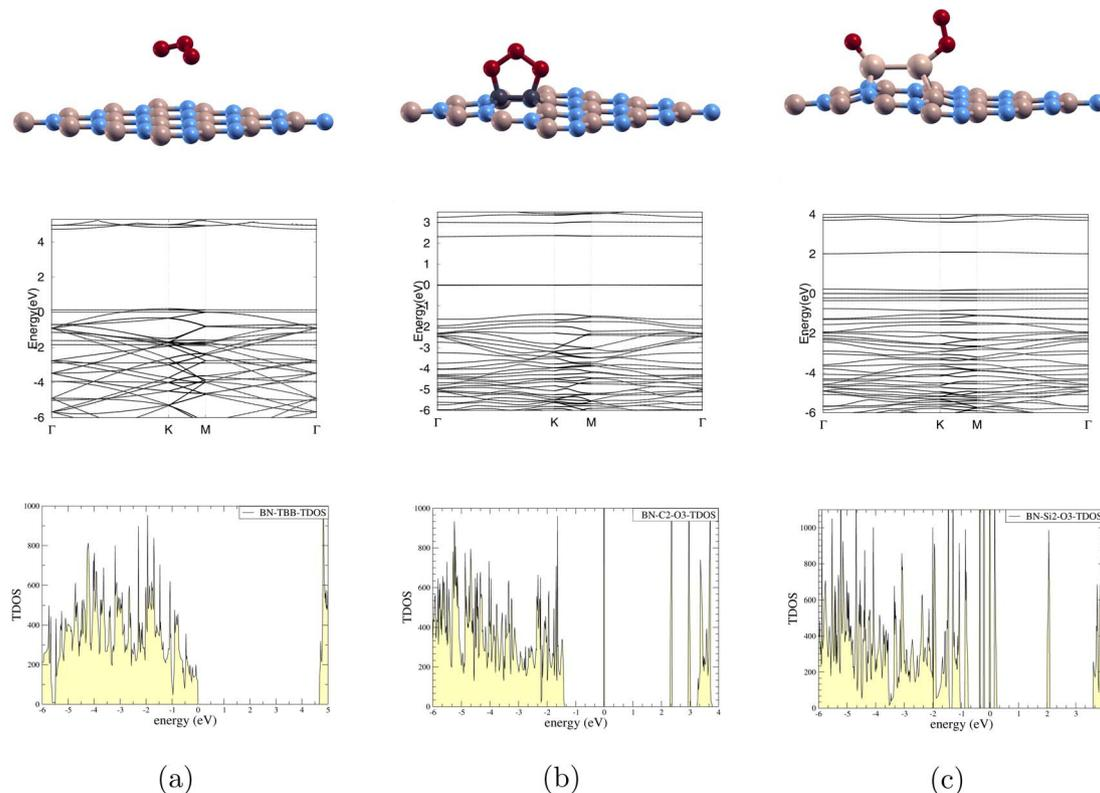
Fig. 5 Ozone adsorbed on monolayers: top row shows side view of atomic structures, middle row shows band structure, and bottom row shows total density of states. 0 eV is Fermi level. (a) BN-T<sub>BB</sub>, (b) O<sub>3</sub>/C-BN, (c) O<sub>3</sub>/Si-BN.
