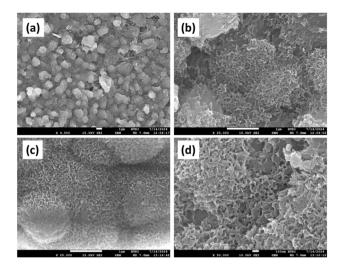
Fig. 15 Bioactivity assessment of the HAp samples after 3 weeks of immersion in SBF solution at 37 °C: (a) and (b) I-HAp and (c) and (d) R-
