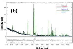
Fig. 2 Rietveld refinement of XRD patterns of (a) I-HAp and (b) R-HAp.
