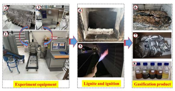
Fig. 1 Experimental apparatus and physical simulation experimental process of lignite underground gasification ((1) the physical simulation apparatus for underground lignite gasification; (2) gasifier; (3) electric simulation steam generator; (4) gasified lignite; (5) syngas firing; (6) char; (7) syngas; (8) Tar).
