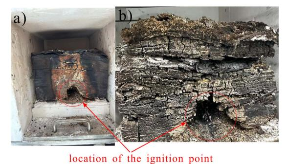
Fig. 3 Position of the ignition point (a) denotes the state of lump coal prior to the gasification reaction; (b) signifies its form subsequent to the
