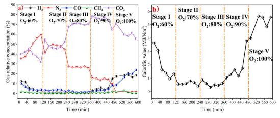
Fig. 6 Characteristics of the syngas and calorific value in the underground coal gasification experiment: (a) characteristics of the syngas, (b) characteristics of calorific value.
