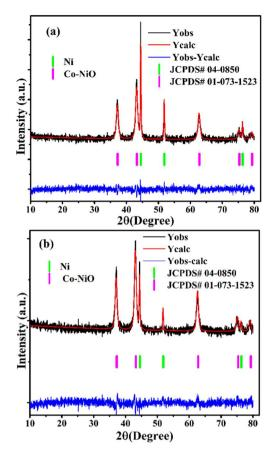
Fig. 4 X-ray diffraction pattern of (a) 20% Co doped Ni/NiO (b) 30% Co doped Ni/NiO nanocomposites. The experimental profile (black) and a full profile matching refinement (red), with the difference given by the blue line of corresponding samples.
