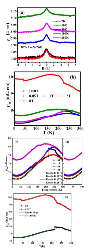
Fig. 3 (a) Magnetoresistance, (b–e) upturn of the electrical resistivity at low temperatures fitted with theoretical data and experimental data for 30% Co-doped Ni/NiO.
