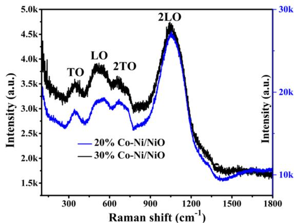
Fig. 5 Raman spectra of the 20% Co and 30% Co-doped Ni/NiO nanocomposites.
