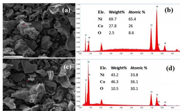
Fig. 7 (a and c) SEM image and its (b and d) point EDS spectra of 20% and 30% Co doped Ni/NiO nanocomposites respectively.
