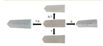
Surface appearance of WUHPC after corrosion.
