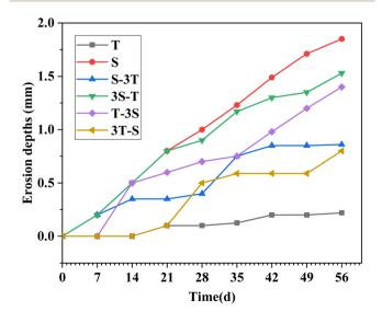
Fig. 8 Erosion depth of WUHPC under different paths.
