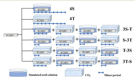
Fig. 2 Schematic of different coupling corrosion regimes.
