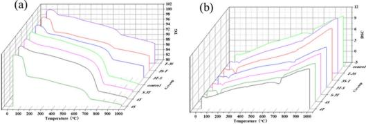
Fig. 10 (a) TG and (b) DSC curves of WUHPC with different corrosion
