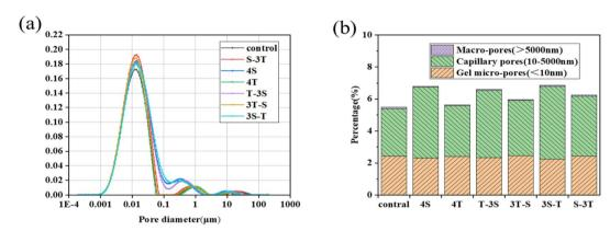
Fig. 11 Effect of different paths on (a) pore size distribution and (b) percentage of porosity
