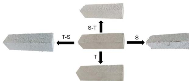
Fig. 6 Surface appearance of WUHPC after corrosion.
