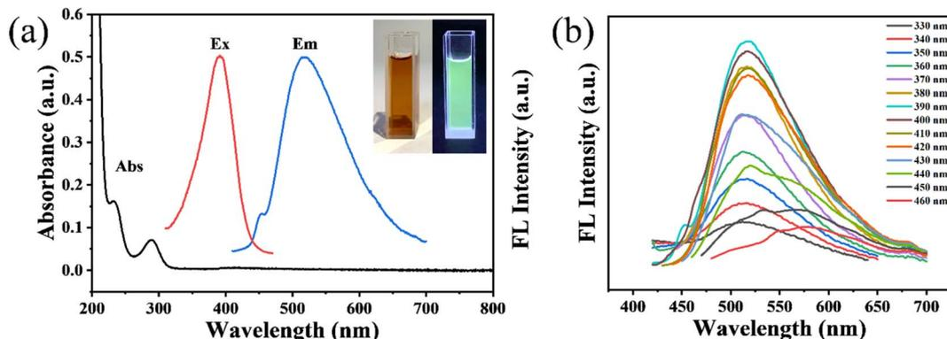
Fig. 3 (a) UV-vis absorption and FL spectra of the GCDs, inset: photos of the GCDs under daylight (left) and UV lamp (right), (b) fluorescence spectra of GCDs at different excitation wavelengths.
