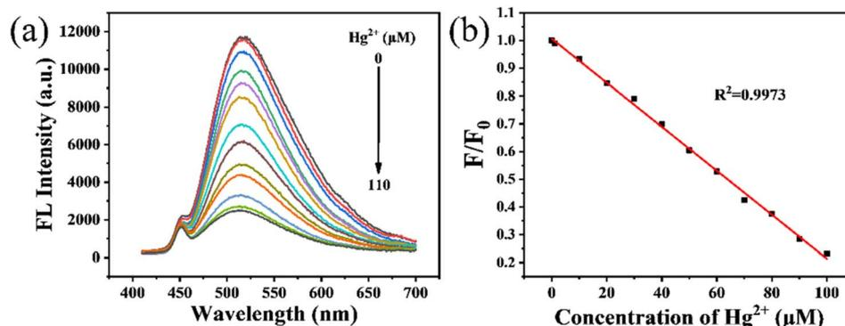
Fig. 5 (a) The fluorescence spectra of the GCDs with different concentrations of Hg<sup>2+</sup> (0–110 μM), (b) the linear relationship between  $F/F_0$  and the concentration of Hg<sup>2+</sup>.
