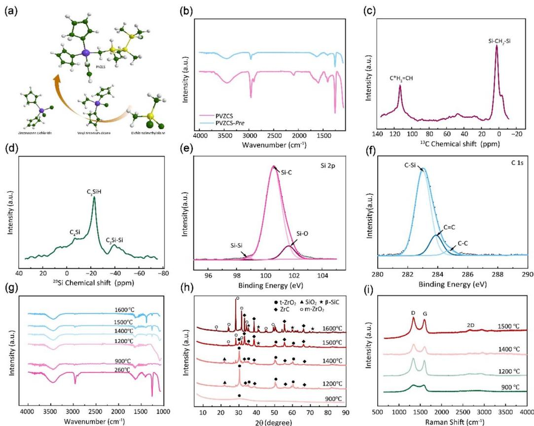
Fig. 2 (a) Schematic illustration of the preparation process of PVZCS. (b) FTIR infrared spectroscopic analysis of PVZCS and PVZCS-Pre. (c) Nuclear magnetic resonance spectroscopy spectrum of  $^{13}\text{C}$ -NMR and (d) spectrum of  $^{29}\text{Si}$ -NMR for the molecular. (e) Si 2p XPS spectrum and (f) C 1s spectra of indicated PVZCS. (g–i) FTIR spectra, XRD pattern and Raman plot of the specimen subjected to pyrolysis and annealing at temperatures ranging from 900 °C to 1600 °C.
