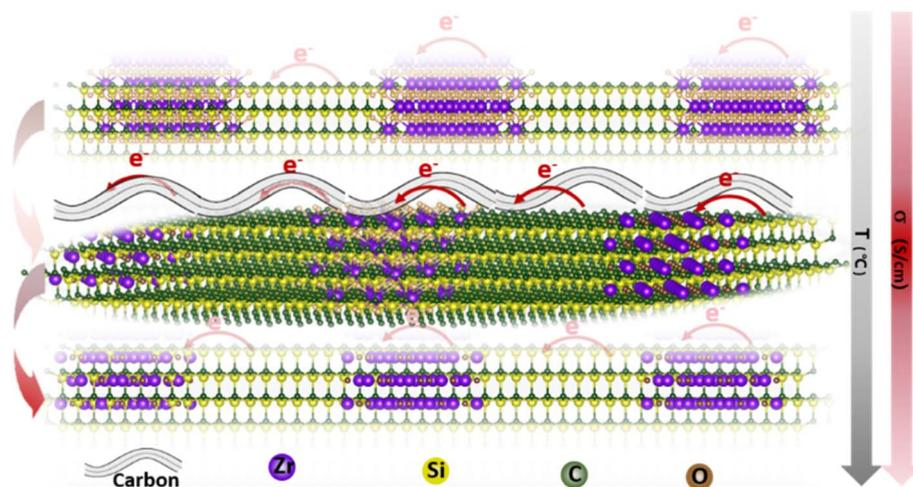
Fig. 1 Schematic illustration of the electron transport route within the SiC-based ceramics under different formations.
