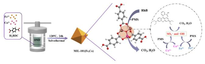
Fig. 9 The schematic shows the synthesis of MIL-101(Fe,Co) and its dye degradation mechanism. From ref. 163 with permission. Copyright 2023, Elsevier.
