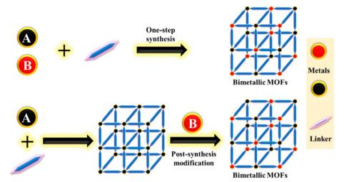
Fig. 6 Illustration of synthesis strategies for BMOFs using one-step and post-synthetic approaches
