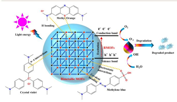
Schematic diagram of dye adsorption and degradation.
