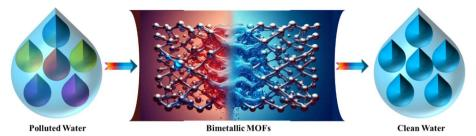
Fig. 2 Schematic diagram depicting BMOFs for dye removal.
