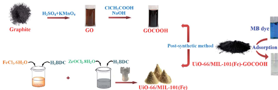
Fig. 7 Diagram showing the synthesis of the composite and images illustrating the adsorption process. From ref. 139 with permission. Copyright 2020, Royal Society of Chemistry.
