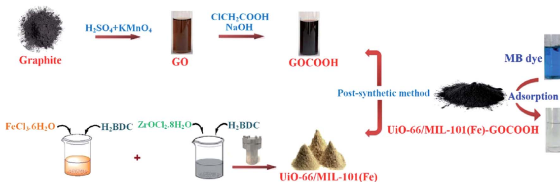
Fig. 7 Diagram showing the synthesis of the composite and images illustrating the adsorption process. From ref. 139 with permission. Copyright 2020, Royal Society of Chemistry.
