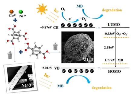
Diagram of sample synthesis and photocatalytic mechanism. Form ref. 140 with permission. Copyright 2022, Elsevier.
