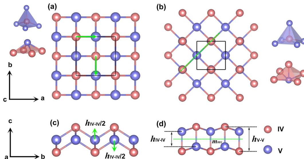
**Fig. 1** (a and c) Top and side views of 2D group IV–V monolayers in the Td3 phase, (b and d) corresponding ones for the Td4 phase. The group IV- and V-atom centered polyhedrons are shown in the left panel of (a) for the Td3 phase, and shown in the right panel of (b) for the Td4 phase. The green arrows in (a) and (c) illustrate the transformation from the Td3 phase to the Td4 phase. The green dashed lines in (b) and (d) indicate the glide line and the mirror plane respectively.
